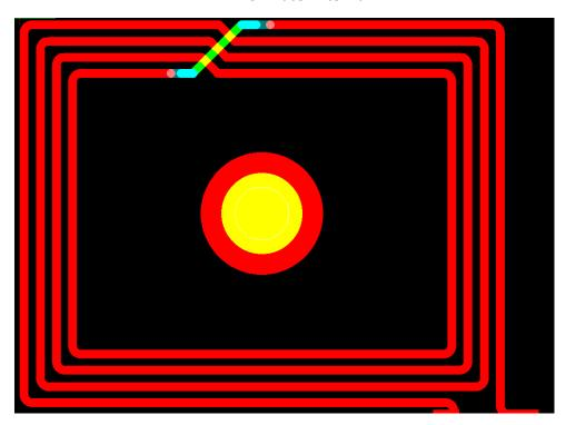
RFID PCB Trace antenna on 00095-002 Antenna dimensions: 30.4mm by 24mm 4 Turns with 20 mil trace width and 20 mil trace spacing 25 ohm single ended impedance Tuned to 25 ohms @ 13.56 MHz
