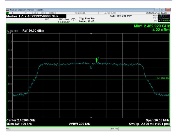
$RF\ Antenna\ Conducted-High\ Channel-802.11n-Reference\ Level-RedPine$
