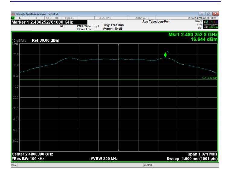
$RF\ Antenna\ Conducted-High\ Channel-BLE-Reference\ Level-Nordic$
