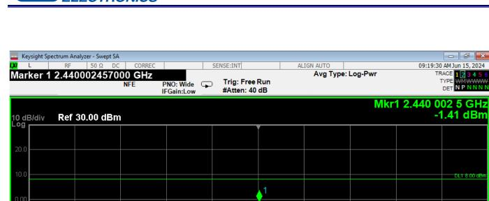
Peak Power Spectral Density - Middle Channel - BLE Mode - RedPine
