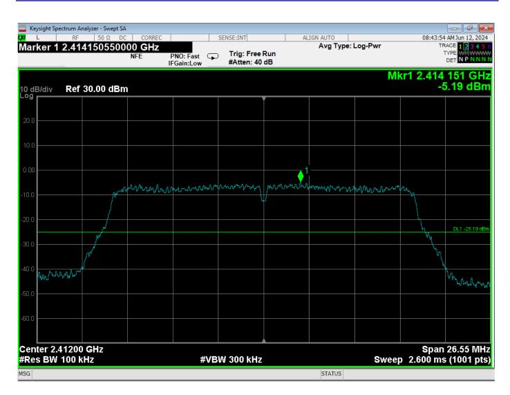
RF Antenna Conducted - Low Channel - 802.11n - Reference Level - RedPine
