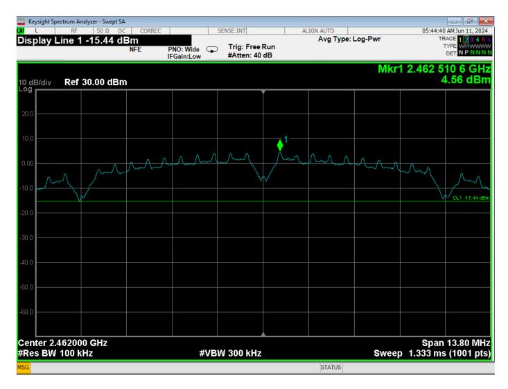
RF Antenna Conducted - High Channel - 802.11b Mode - Reference Level - RedPine
