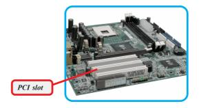
**Step 2.** Put the PC54G (MS-6825) directly over the PCI slot and press it into the slot firmly.
