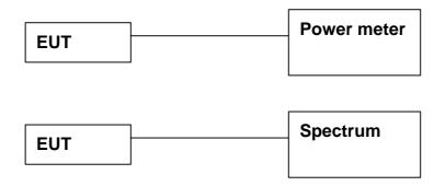
The EUT was connected to a spectrum through a 50 RF cable.
