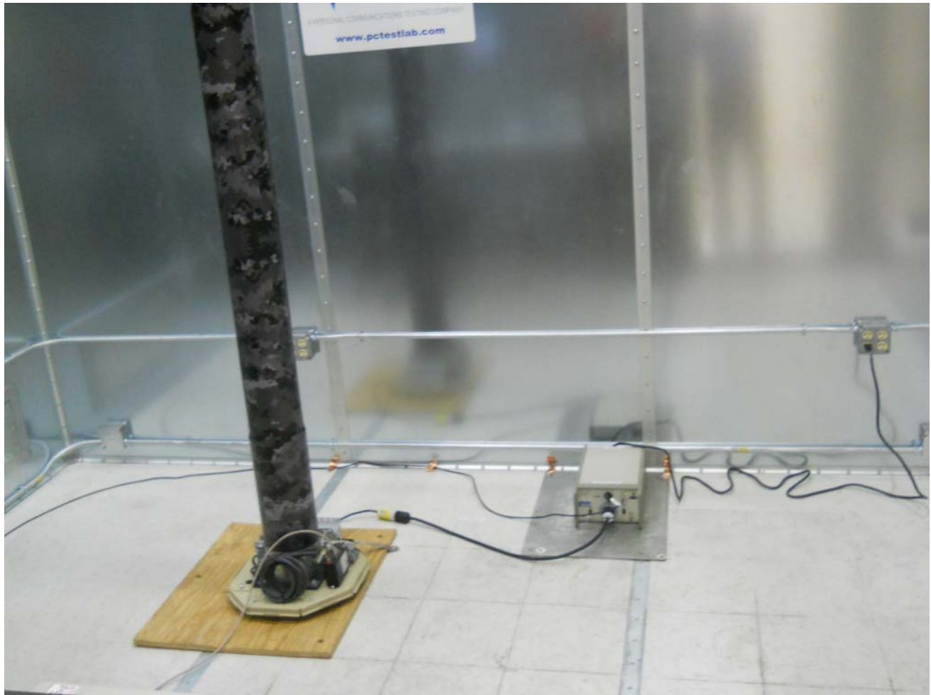
Figure 1. AC Line Conducted Test Setup
