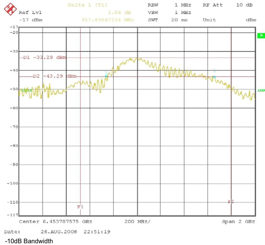
**5.0 15.250(a) and 15.250(b): -10 dB Bandwidth requirements (Bandwidth)****Data:**
