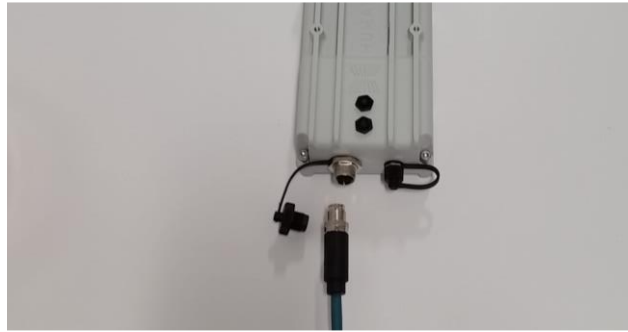
Fig. 12: Illustration of POE cable to Beacon connection.
