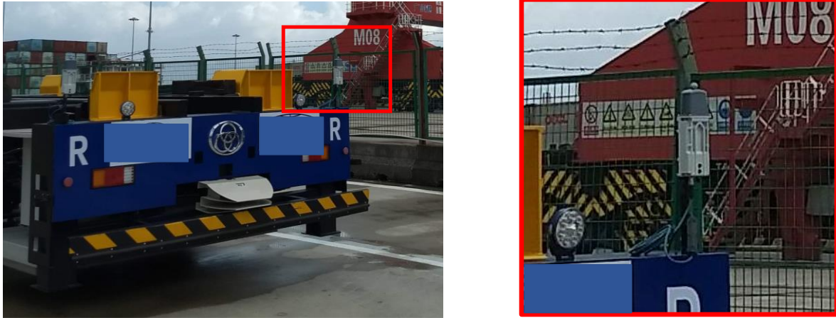
Fig. 9: Beacon mounted on beam above rear corner of vehicle (left) detail (right).
