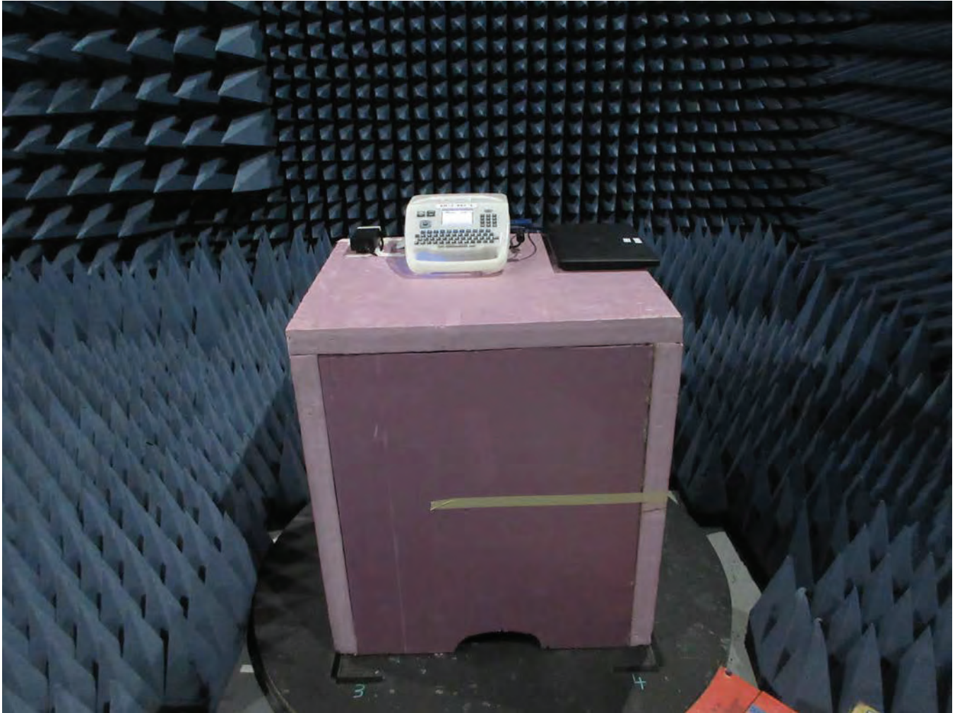
Radiated Above 1 GHz - Front
