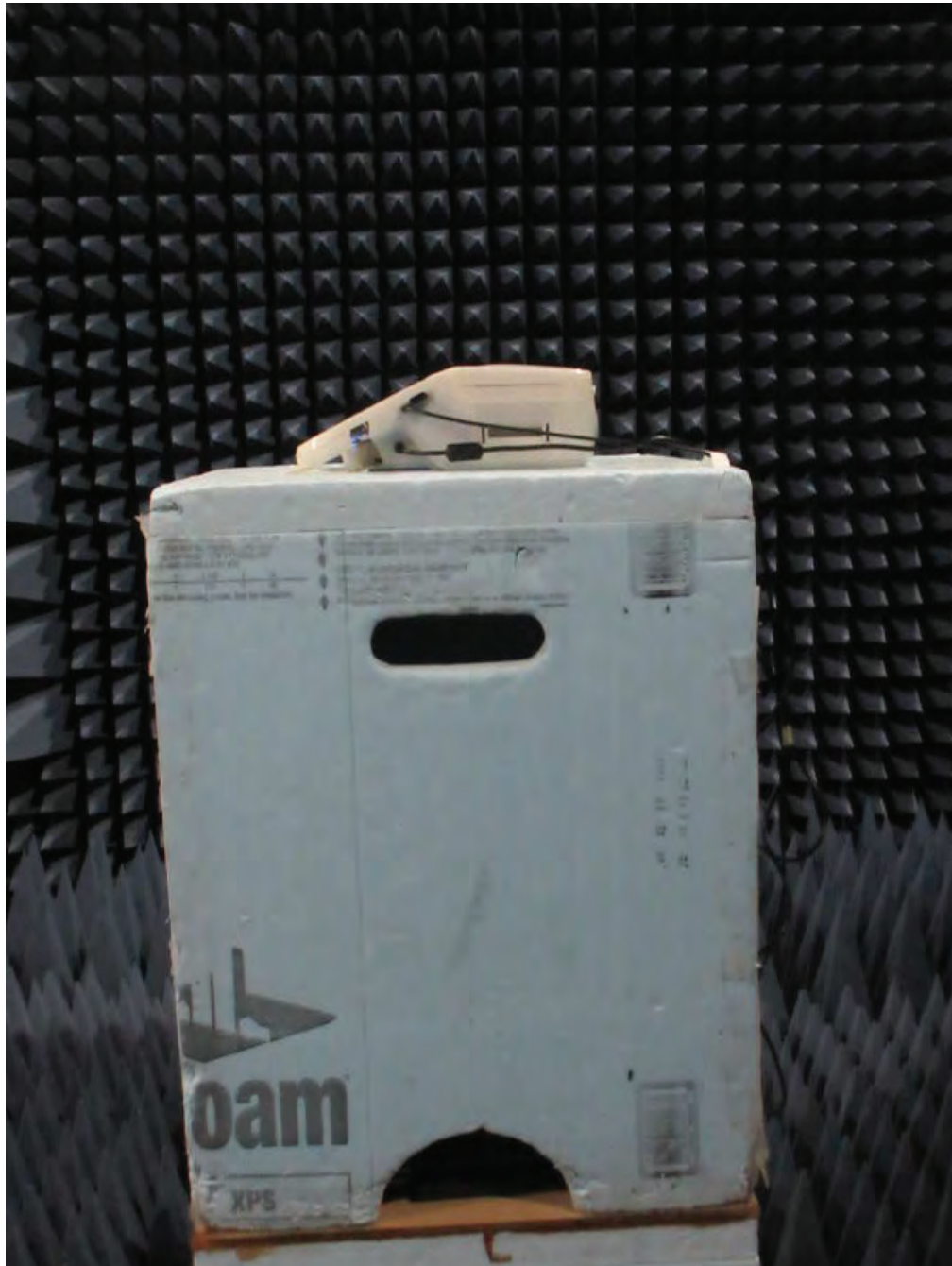
Radiated Above 1 GHz - Side
