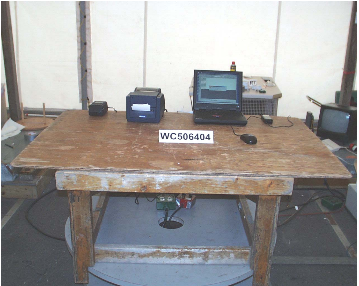
Test-setup photo, radiated emissions
