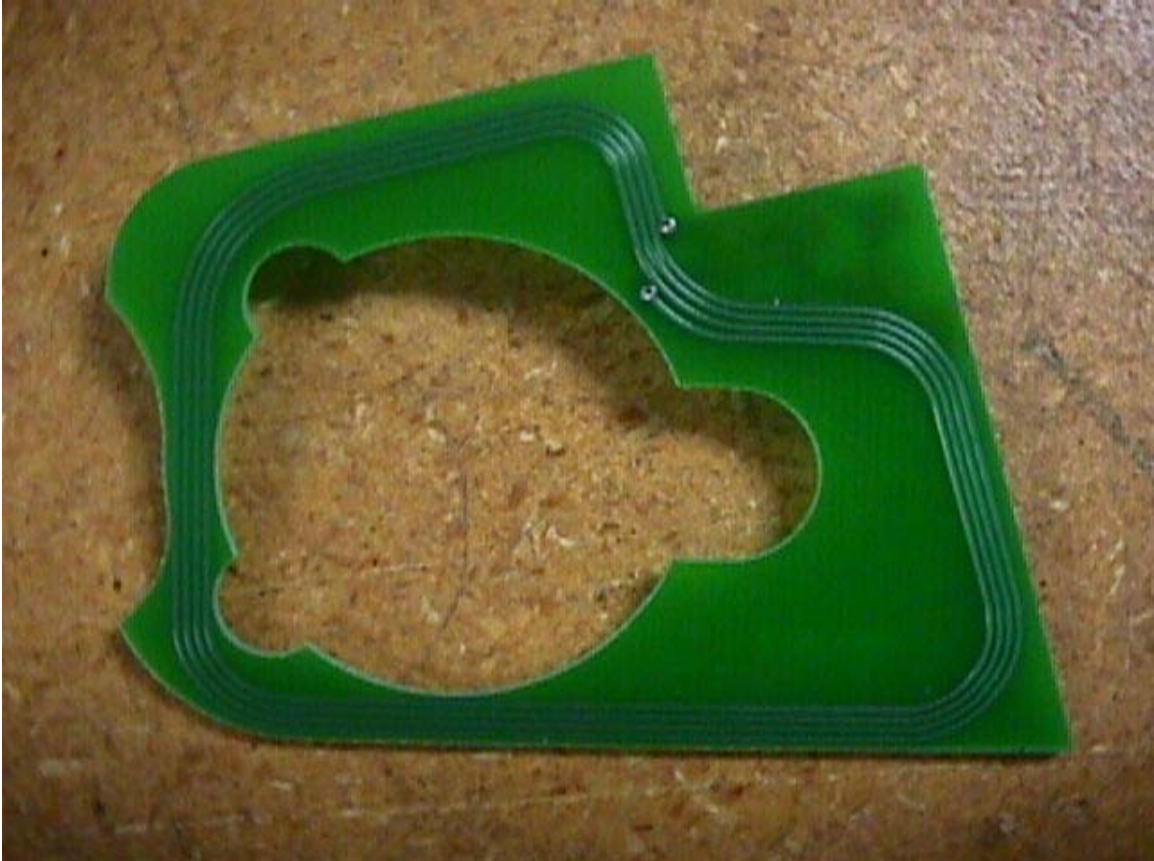
Figure 4 -- Internal view, ribbon antenna - bottom
