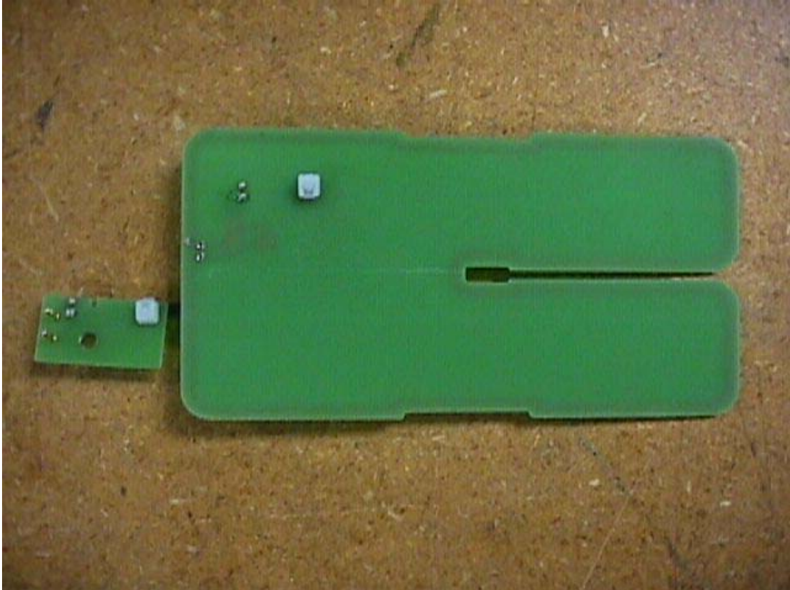
Figure 8 -- Internal view, media antenna and contact board - bottom
