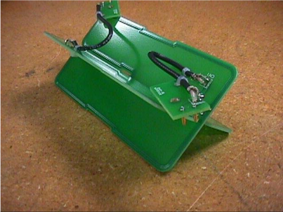
Figure 9 -- Internal view, media antennas and contact boards in X-configuration
