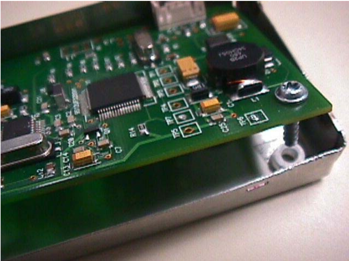
Figure 11 -- Internal view, BDC with metal cover removed
