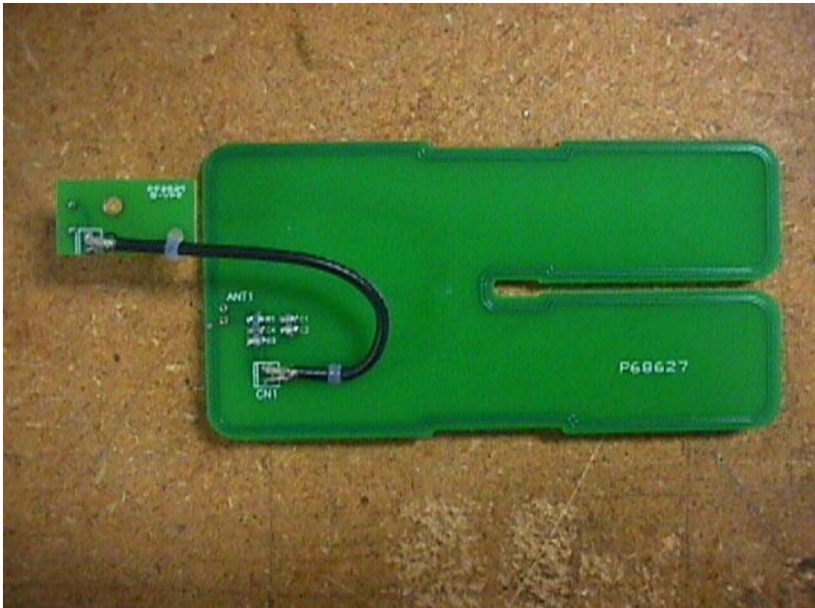
Figure 7 -- Internal view, media antenna and contact board -- top
