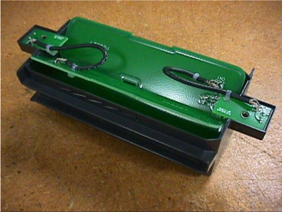
Figure 6 -- Internal view, media antennas in media holder
