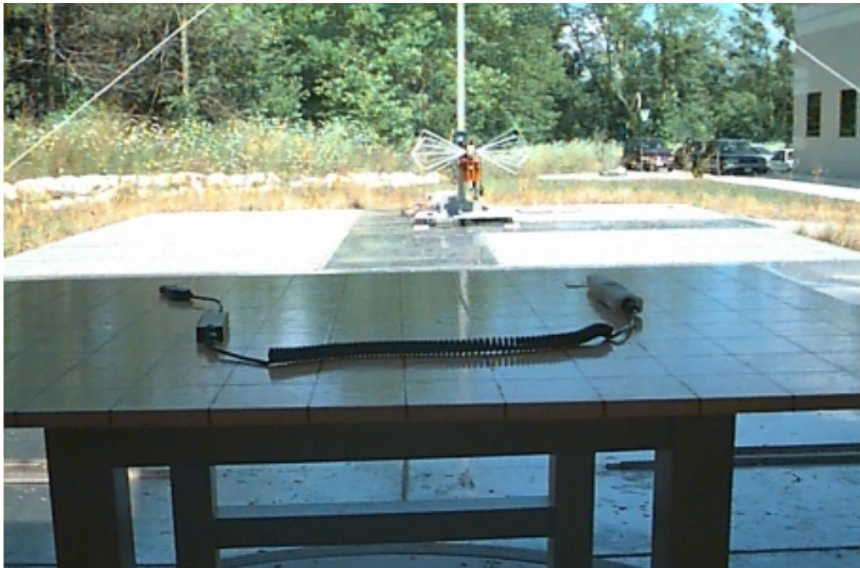
Front view of the Brady portable card reader during the Radiated Emissions tests.
