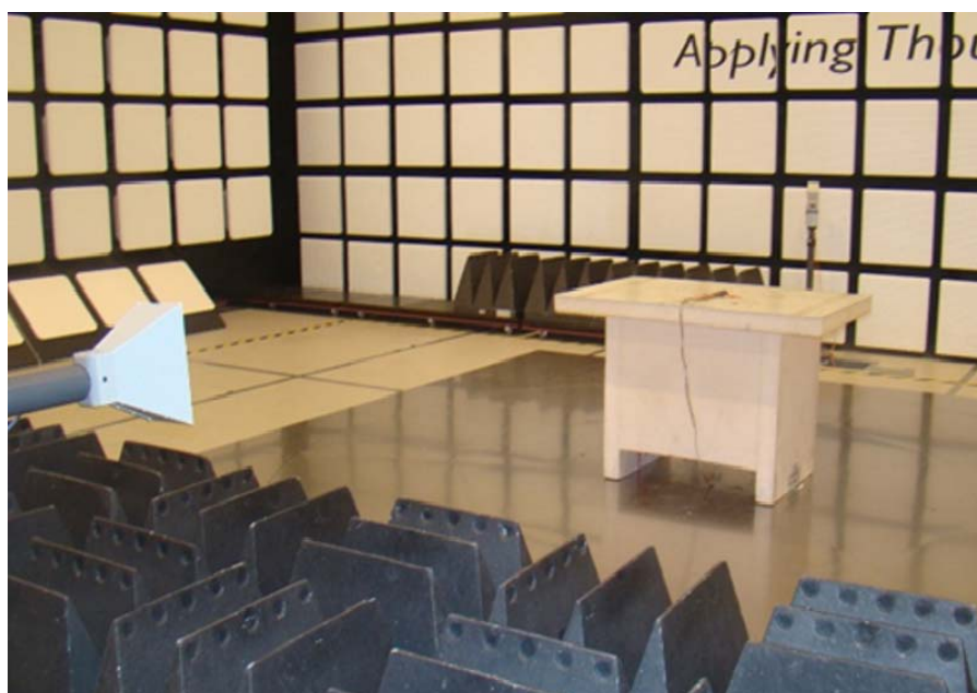
Figure 4: Test setup for Radiated Emission (Horizontal) – 1GHz to 18GHz
