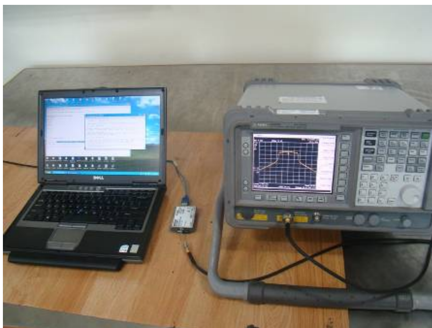
Figure 6: Test setup for Conducted Radio Frequency measurements
