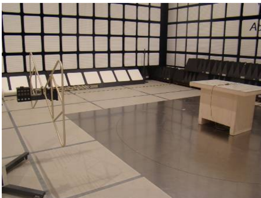
Figure 2: Test setup for Radiated Emission (Horizontal) – 30MHz to 1GHz
