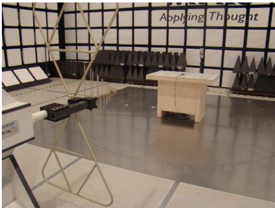
Figure 1: Test setup for Radiated Emission (Vertical) – 30MHz to 1GHz
