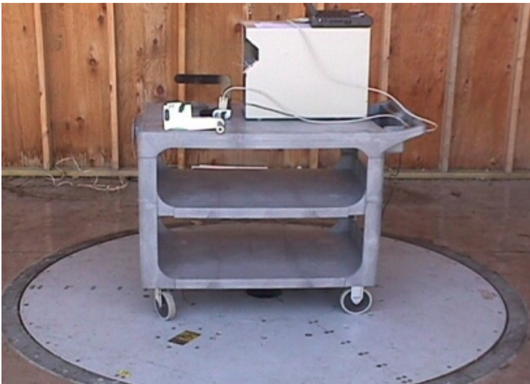
Front view of the Brady EPM during the Radiated Emissions tests.
