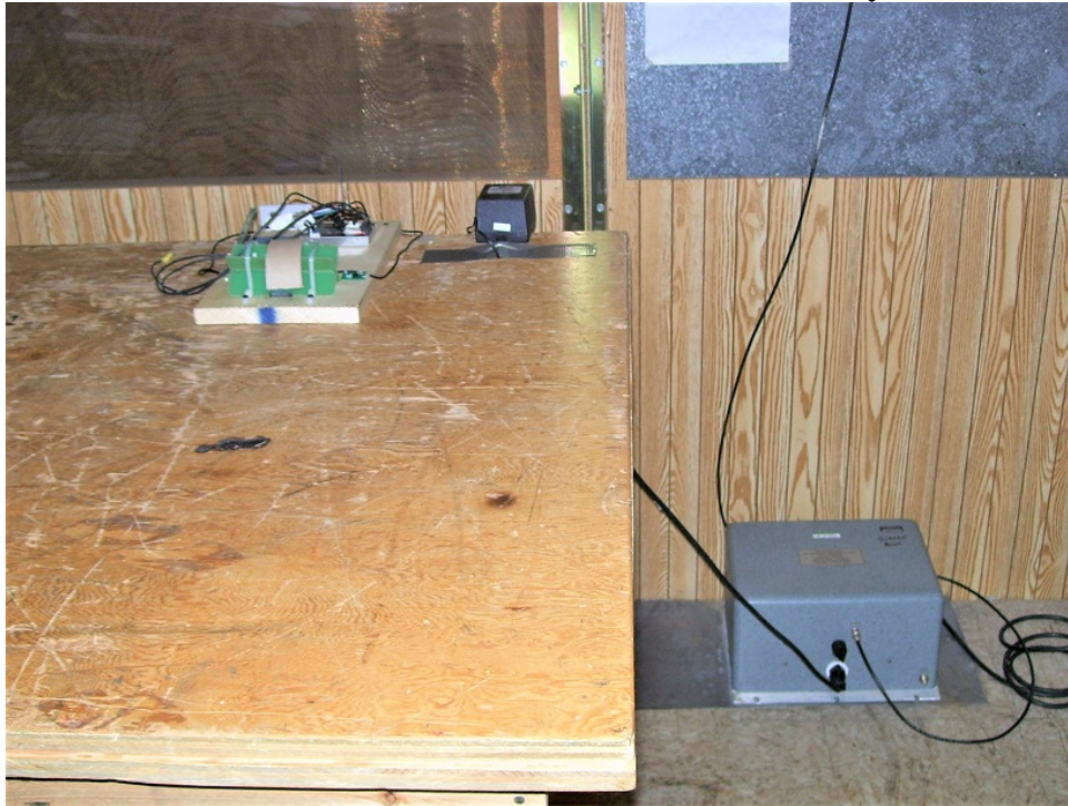
AC line Conducted Emissions – Front with dummy loads
