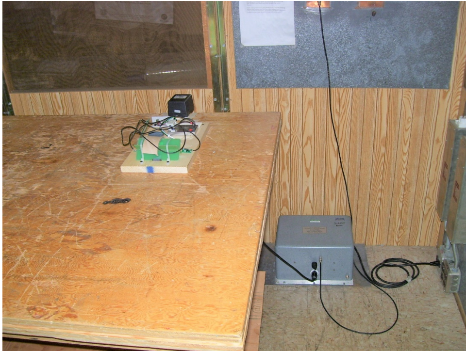
AC line Conducted Emissions – Front with antennas connected
