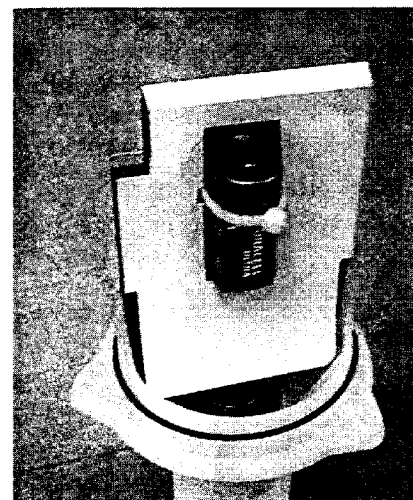
Figure 4. Ultrasonic Monitor without Cover (Replacing the Battery)
