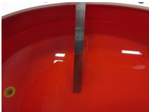
Liquid depth in the flat Phantom ( \geq 15\text{cm} depth) HSL(900MHz)
