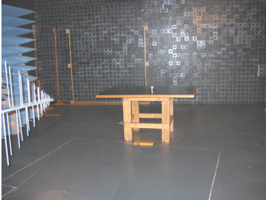
Photograph No.1 Test setup for 6 dB bandwidth measurements and for carrier field strength measurements
