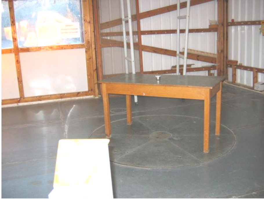
Photograph No.5 Setup for spurious emission field strength measurements at OATS above 1000 MHz
