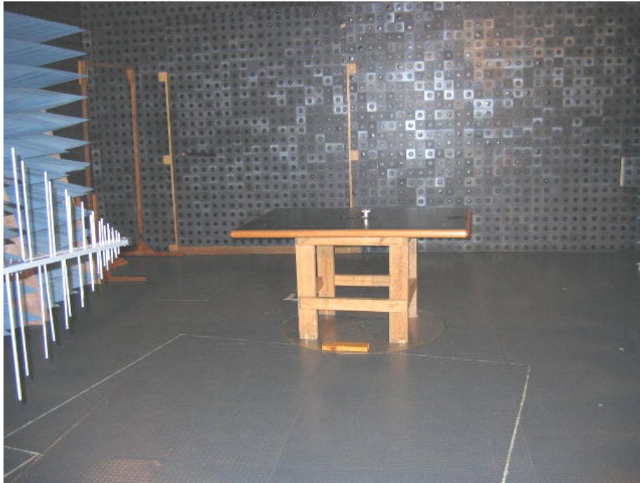
Photograph No.3 Setup for spurious emission field strength measurements in the anechoic chamber from 30 to 1000 MHz and for radiated emission measurements according to §15.109
