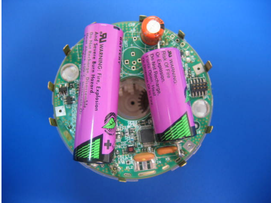
Photograph No.2 ETMW water reader PCB component side with batteries
