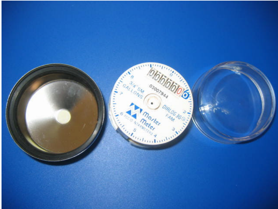
Photograph No.4 ETMW water reader General view with bottom and top enclosures
