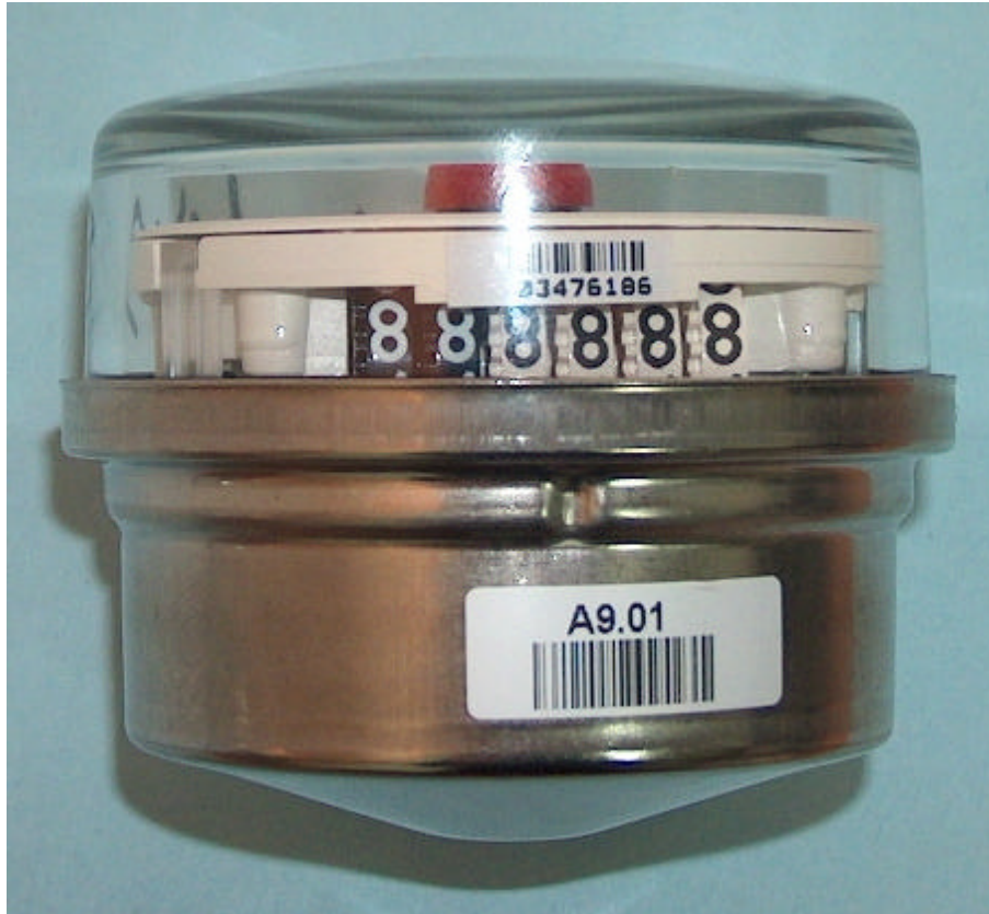
Photograph No.2 ETMW water reader Side view
