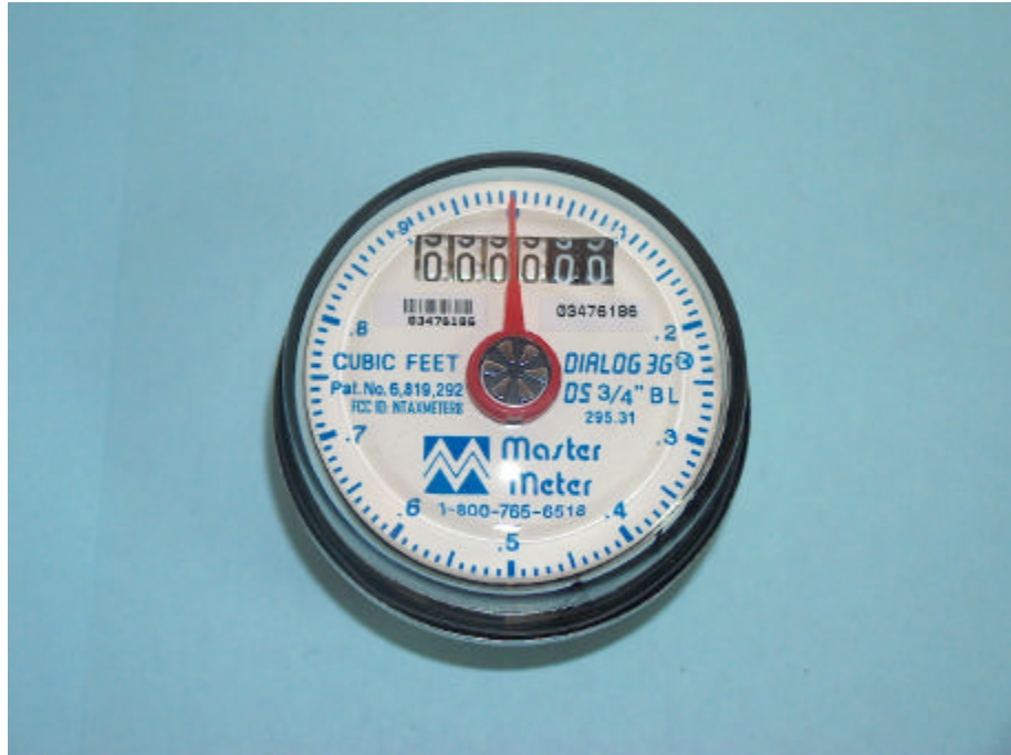
Photograph No.5 ETMW water reader General view without bottom and top enclosures
