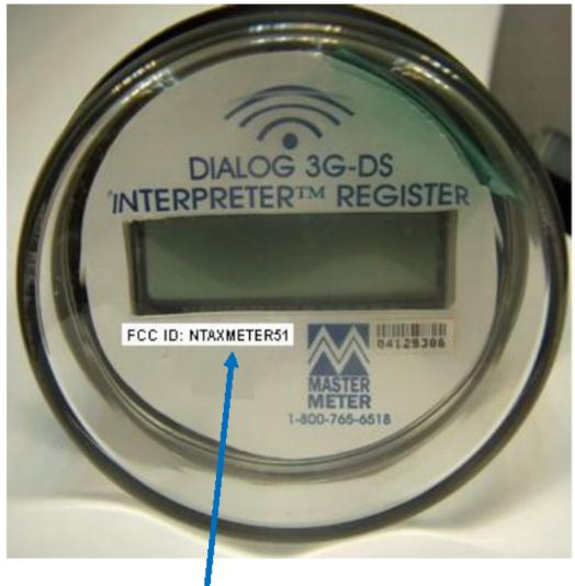
The label with FCC ID:NTAXMETER51 will be located here.
