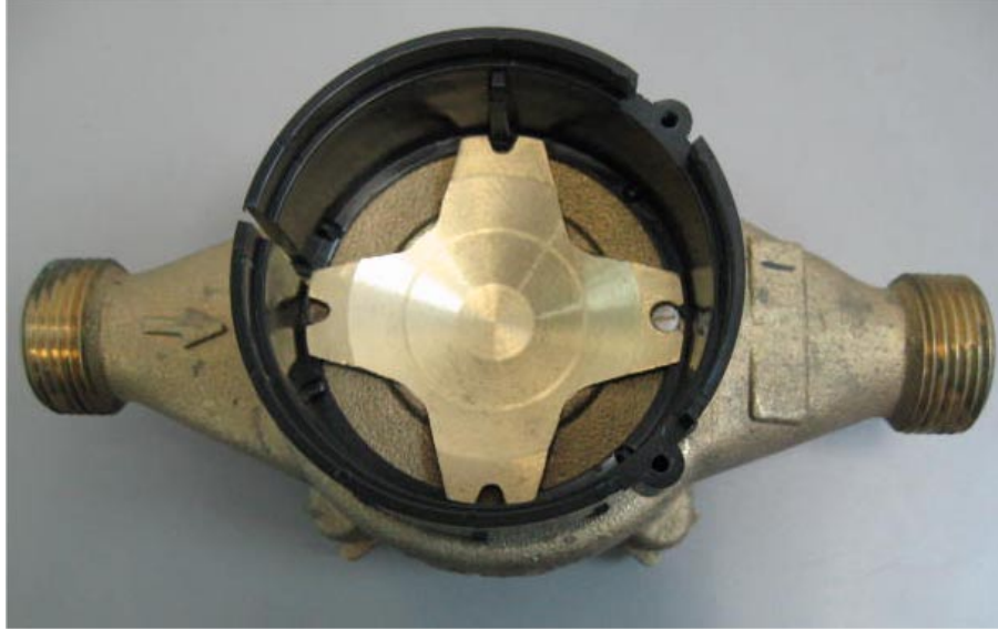
Photograph No.6 DTMW LCD water reader external enclosure
