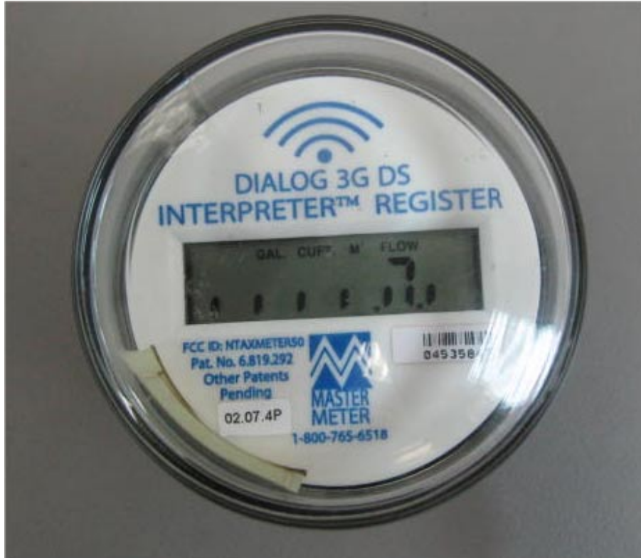
Photograph No.5 DTMW LCD water reader extracted from external enclosure
