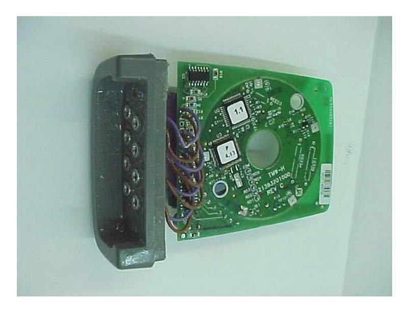
Connection to internal printed antenna
