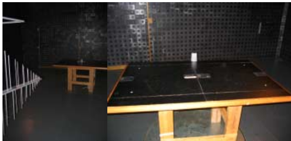
Photograph 7.5.1 Setup for preliminary radiated emission measurements
