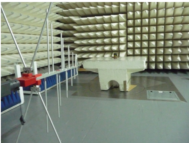
Photograph 8.1.1 Setup for radiated emission measurements
