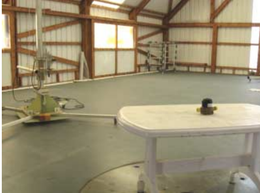
Photograph No.1 Setup for carrier field strength, peak power spectral density measurements at the OATS
