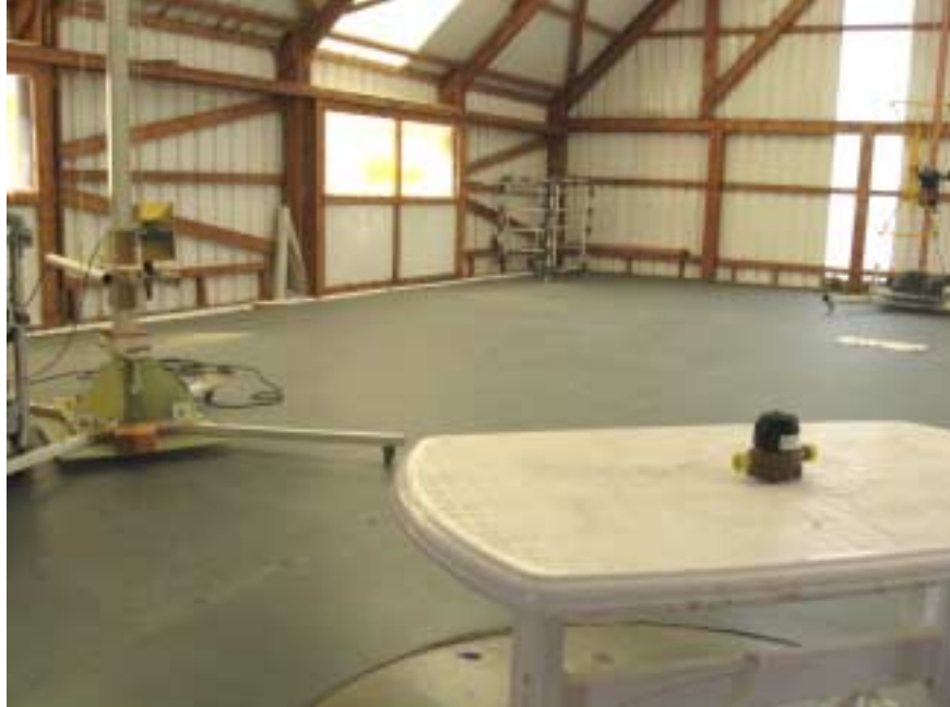
Photograph No.4 Setup for radiated emission measurements at the OATS above 1000 MHz
