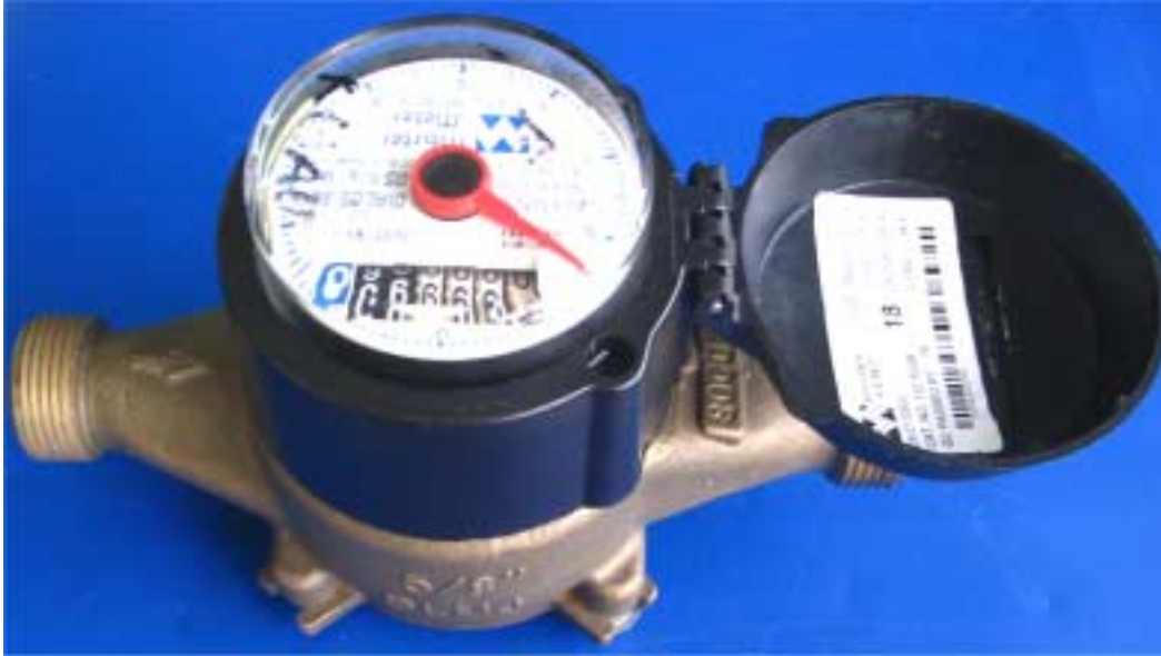
Photograph No.3 DTMW water reader with cover open
