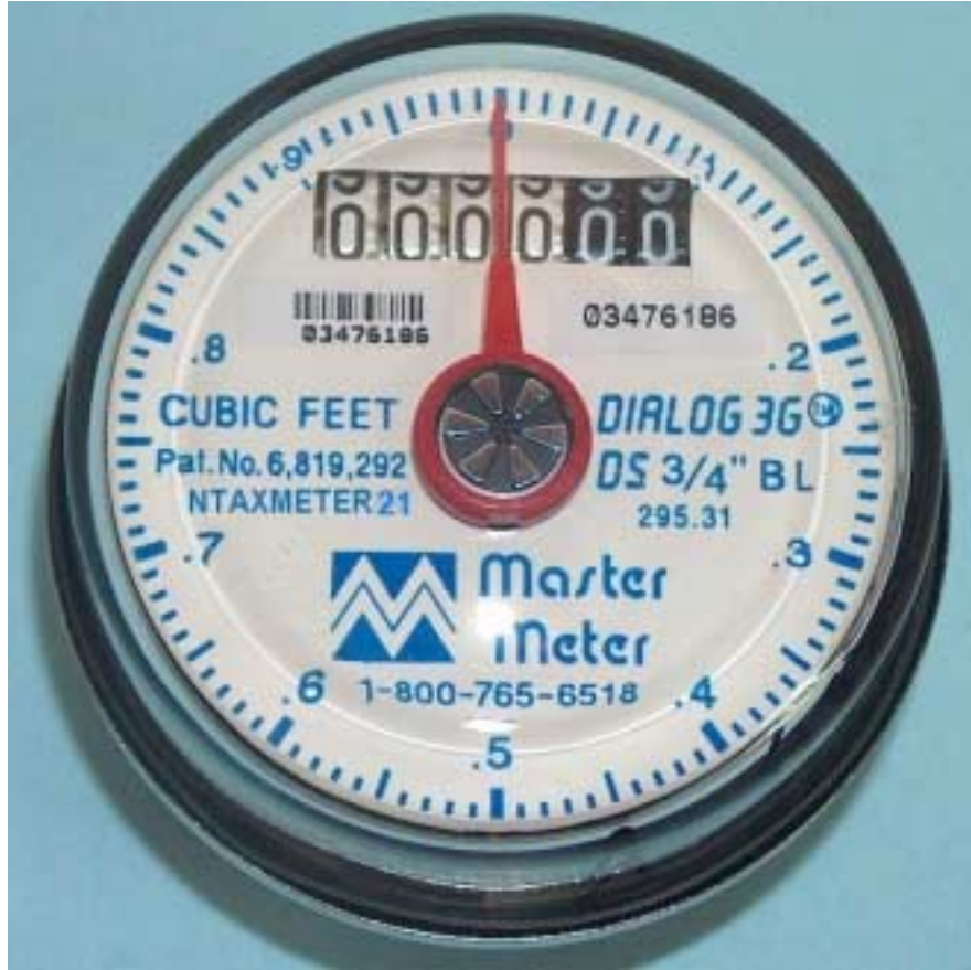
Photograph No.5 DTMW water reader extracted from external enclosure
