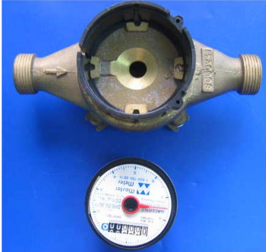
Photograph No.4 DTMW water reader extracted from external enclosure
