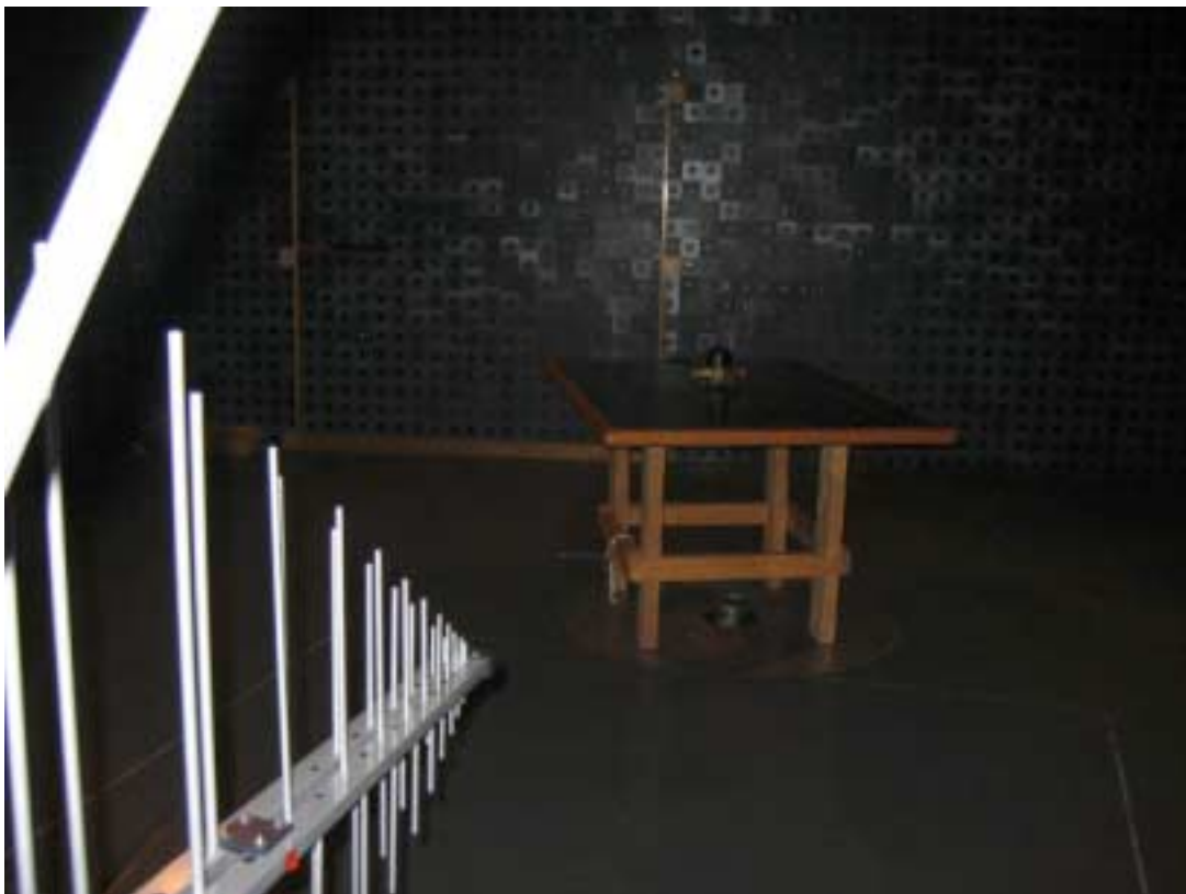
Photograph No.3 Setup for spurious emission field strength measurements in the anechoic chamber from 30 to 1000 MHz
