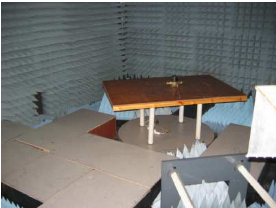
Photograph No.7 Setup for radiated emission measurements from 2900 to 5000 MHz according to §15.109
