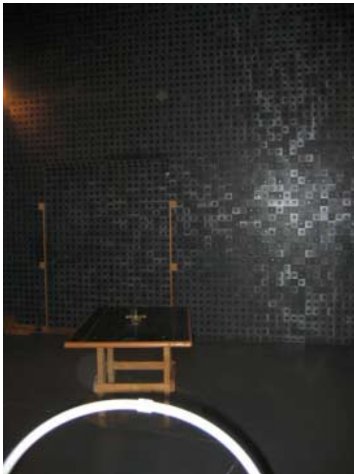
Photograph No.2 Setup for spurious emission field strength measurements in the anechoic chamber below 30 MHz
