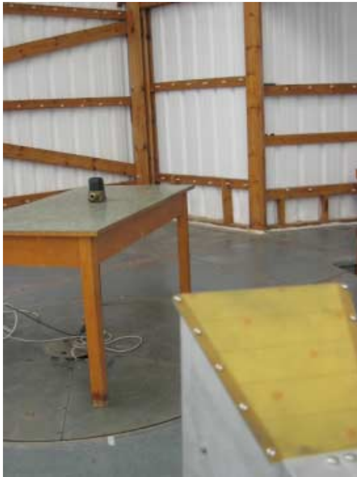
Photograph No.5 Setup for spurious emission field strength measurements at OATS above 1000 MHz
