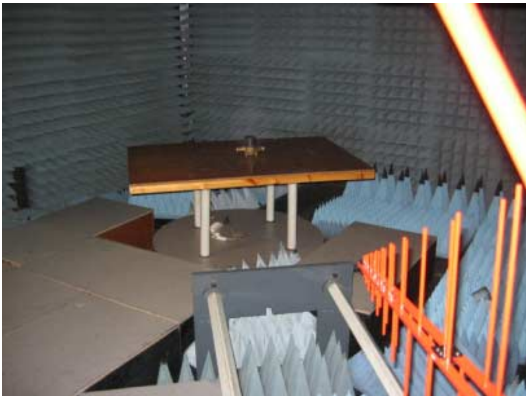
Photograph No.6 Setup for radiated emission measurements from 30 to 2900 MHz according to §15.109
