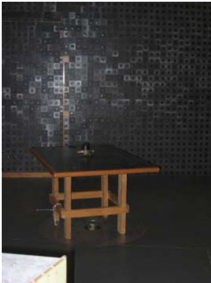
Photograph No.4 Setup for spurious emission field strength measurements in anechoic chamber above 1000 MHz
