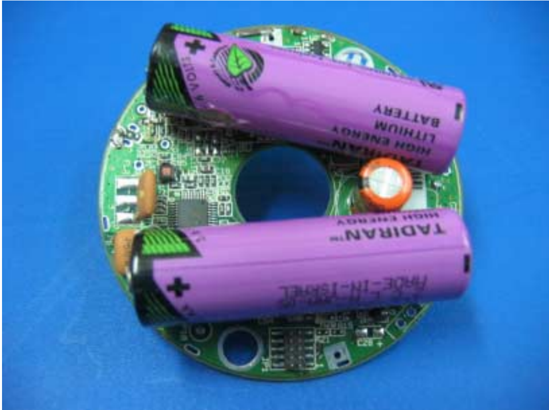
Photograph No.2 ETMW-NA water reader PCB component side with batteries
