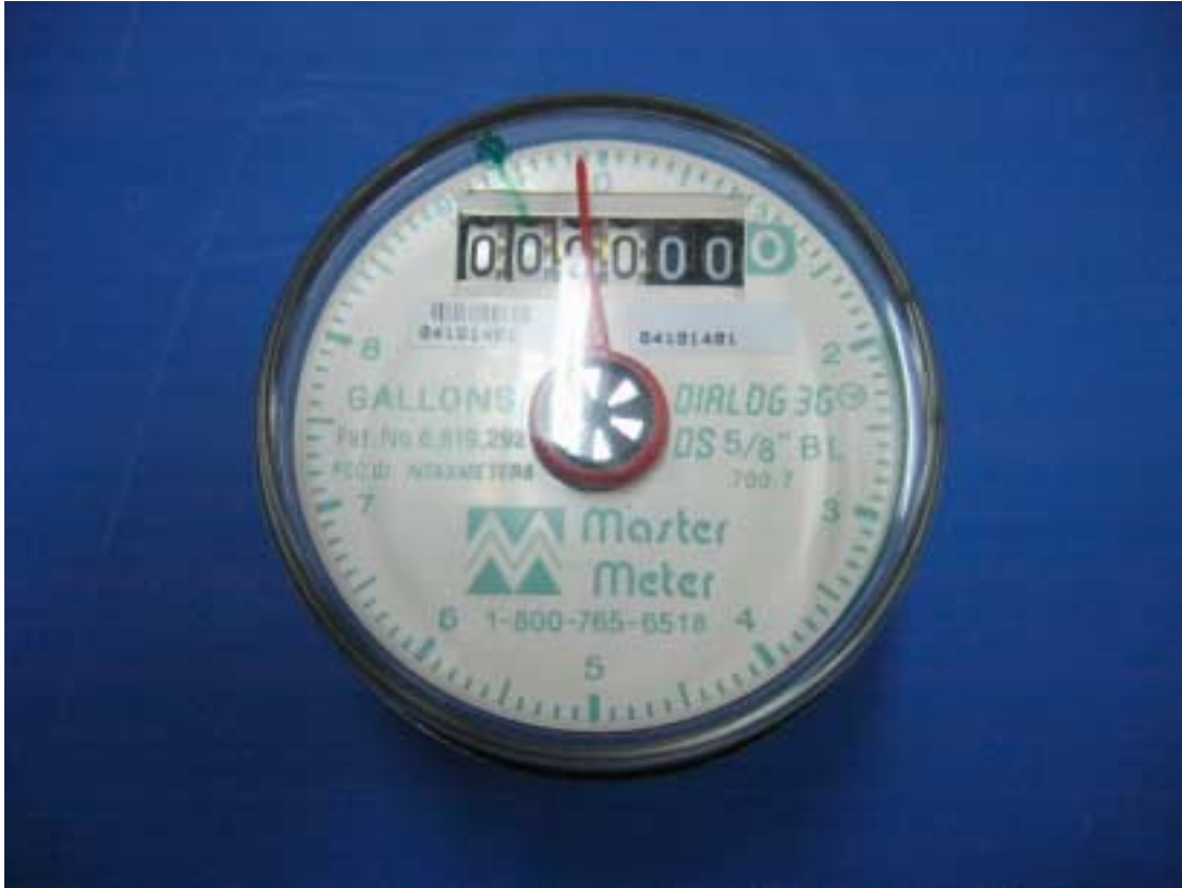
Photograph No.4 ETMW-NA water reader Top view
