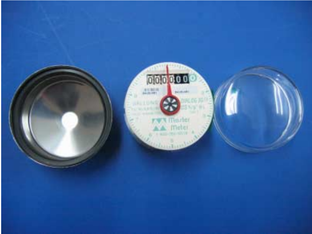
Photograph No.8 ETMW-NA water reader Top view with bottom and top enclosures
