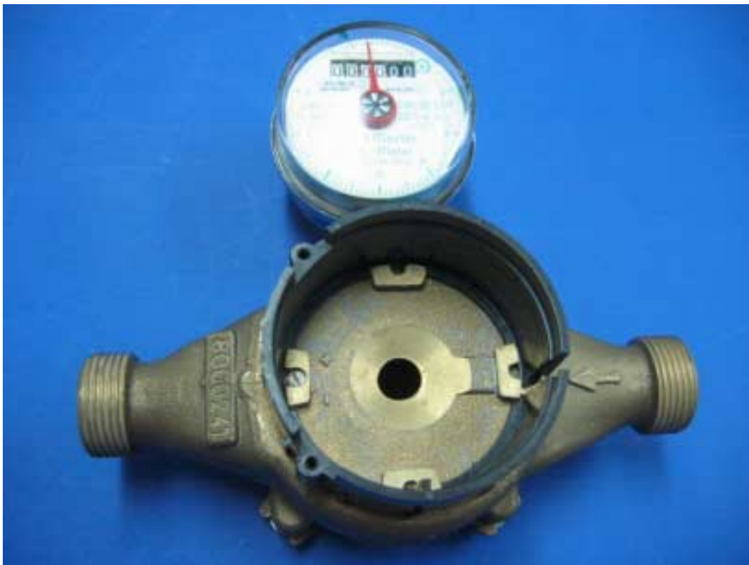
Photograph No.3 ETMW-NA water reader extracted from external enclosure
