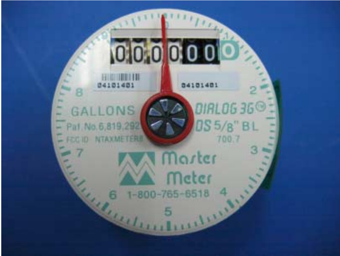
Photograph No.9 ETMW-NA water reader General view without bottom and top enclosures
