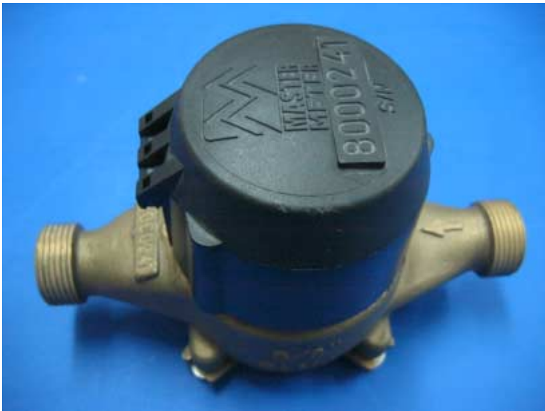
Photograph No.1 ETMW-NA water reader General view with cover closed
