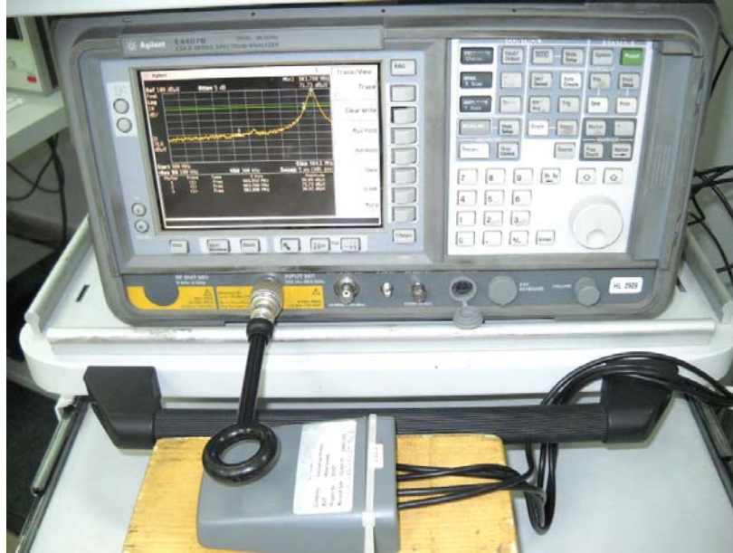
Photograph No.4 Band edge emission test setup
