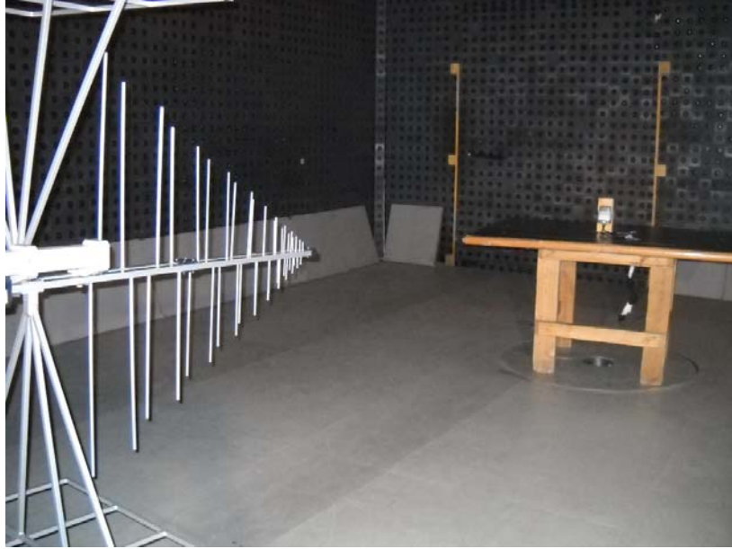
Photograph No.1 Setup for carrier, spurious emissions field strength and OBW measurements in the anechoic chamber from 30 to 1000 MHz
