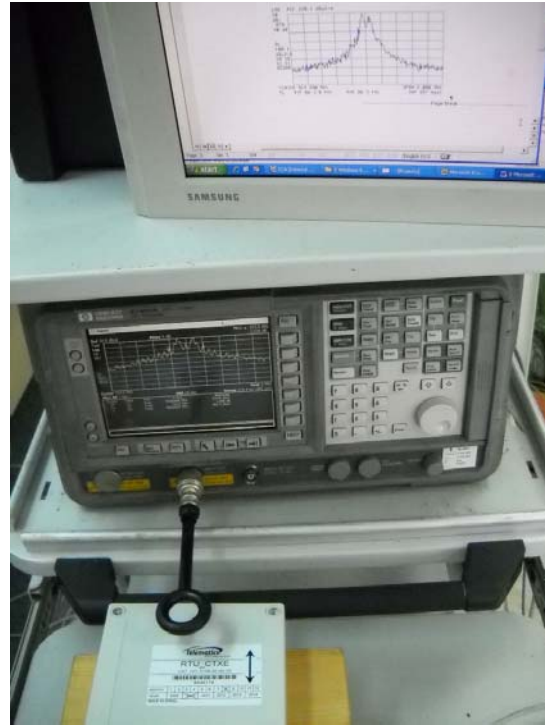
Photograph No.4 Band edge emission, OBW and hopping parameters test setup
