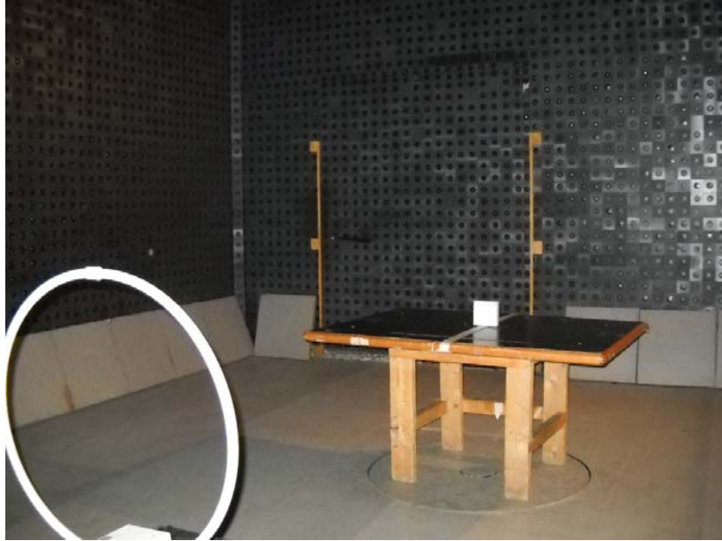
Photograph No.2 Setup for spurious emission measurements in the anechoic chamber below 30 MHz
