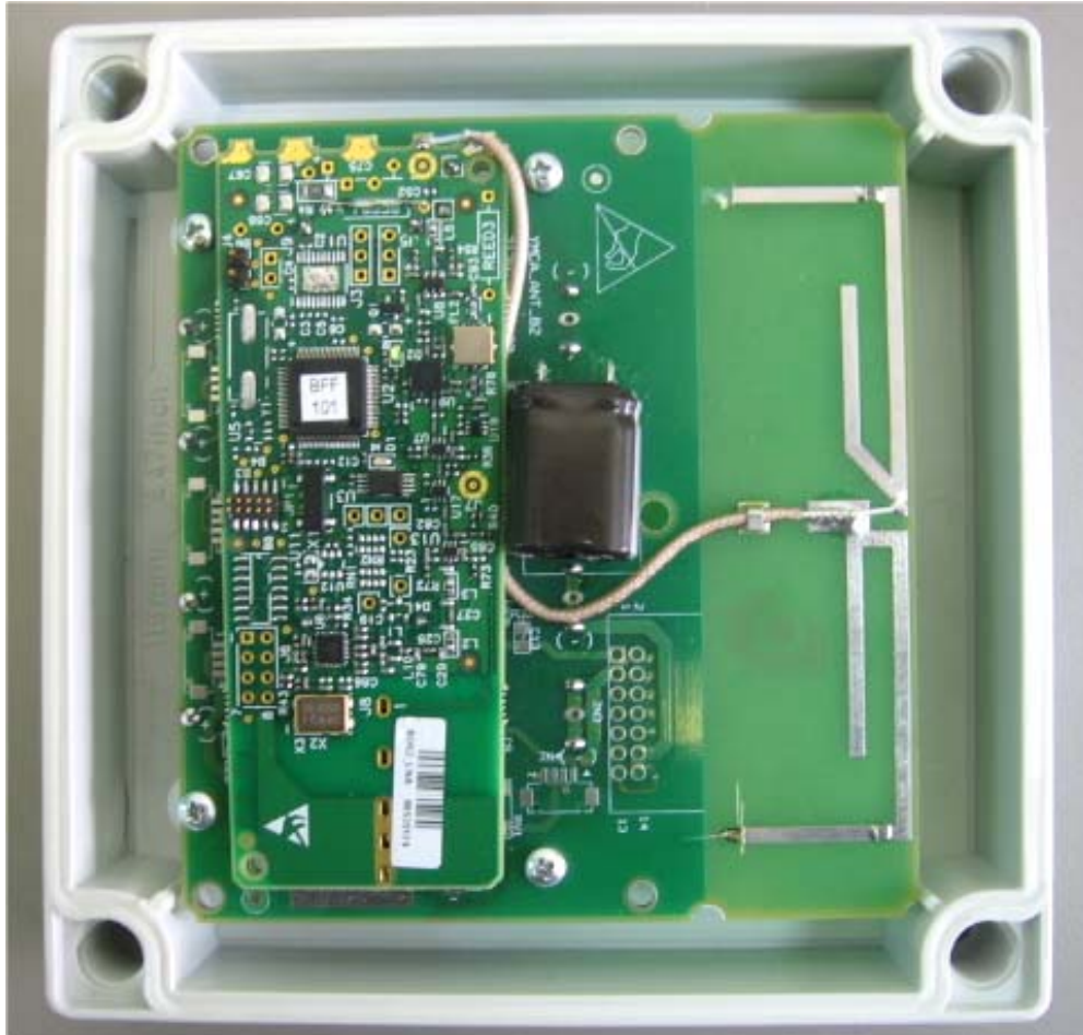
Photograph No.1 WMB booster internal view
