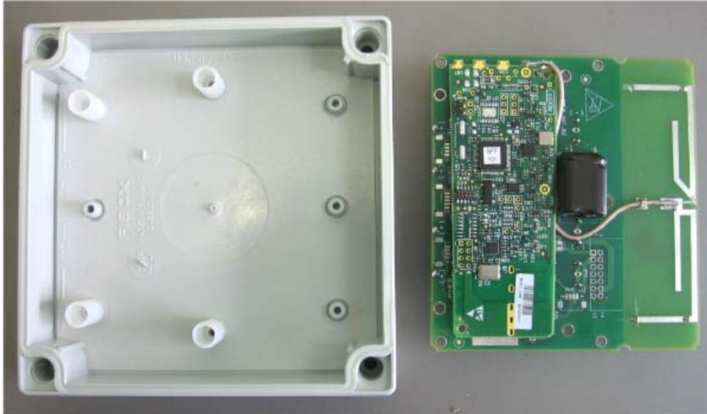
Photograph No.2 WMB booster internal view with PCB removed
