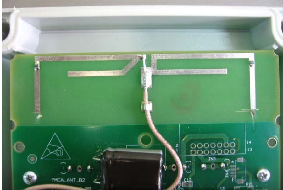
Photograph No.5 Antenna close view
