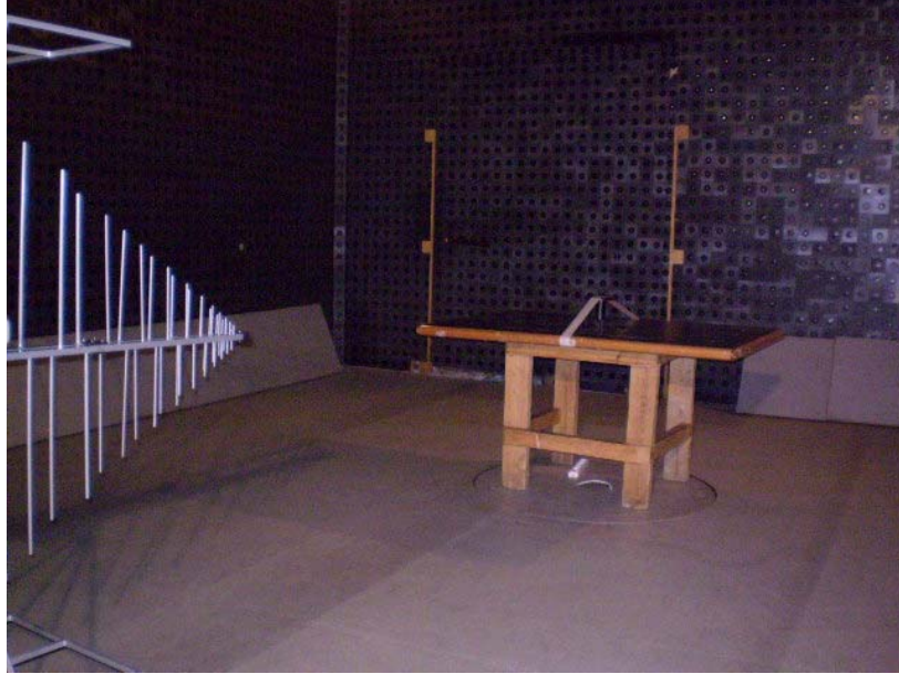
Photograph No.3 Setup for OBW measurements in the anechoic chamber from 30 to 1000 MHz
