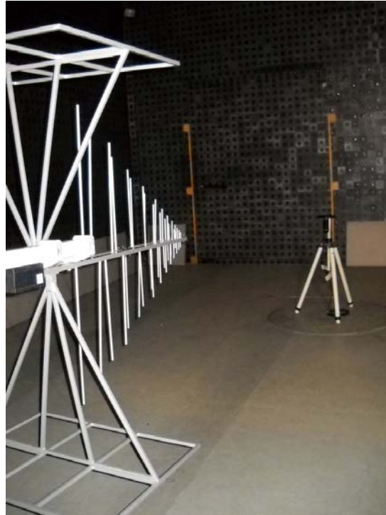
Photograph No.1 Setup for carrier and spurious emissions field strength measurements in the anechoic chamber from 30 to 1000 MHz
