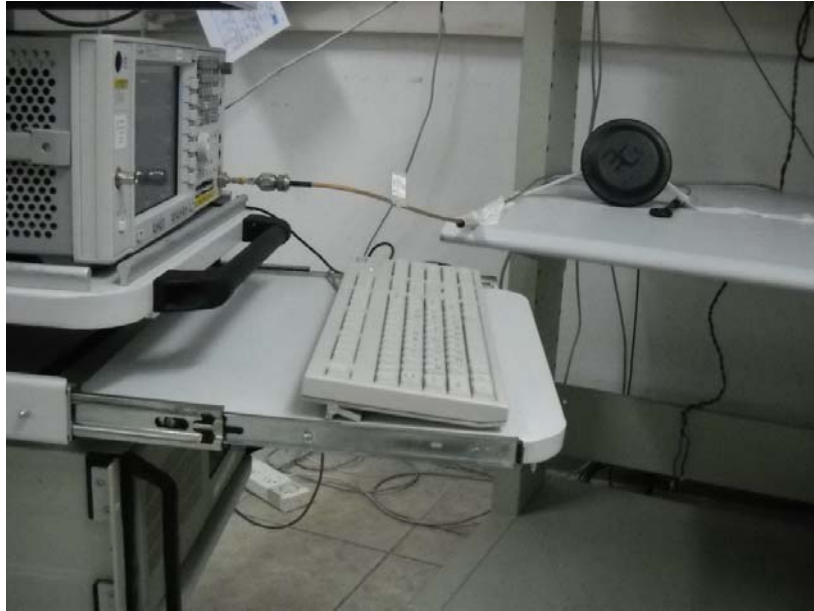
Photograph No.5 Frequency hopping parameters measurement test setup
