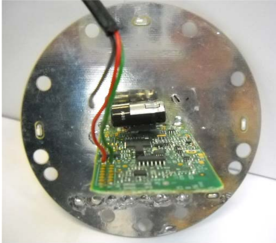
Photograph No.2 2WB-LG booster internal view
