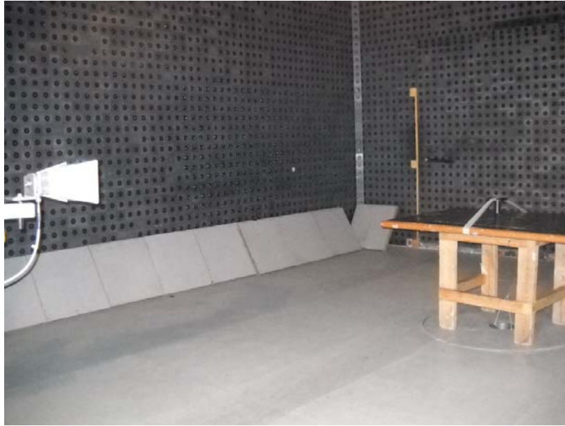
Photograph No.4 Setup for spurious emission measurements in the anechoic chamber above 1000 MHz
