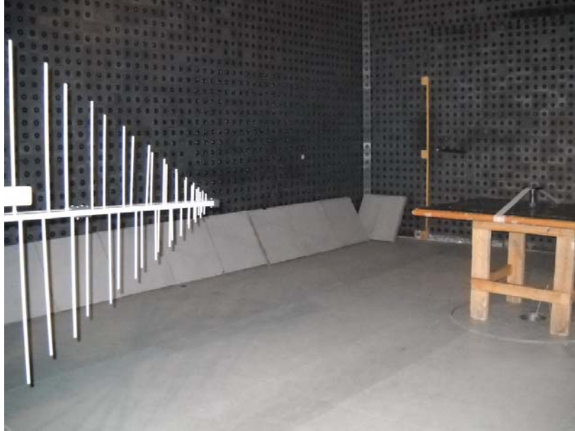
Photograph No.3 Setup for carrier field strength, power spectral density and spurious emission measurements in the anechoic chamber from 30 to 1000 MHz
