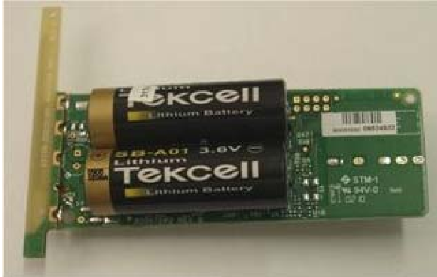
Photograph No.4 Booster 2 PCB with batteries
