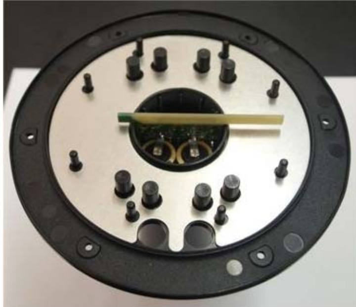
Photograph No.2 Booster 2 integrated OMNI antenna view
