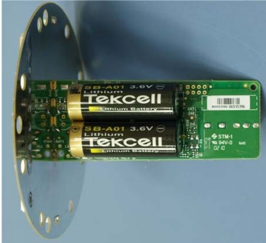
Photograph No.3 Booster 2 internal view with batteries
