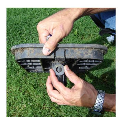
4. Position the assembled Pit-Set Lid with the Booster unit back on the Pit (after the Beep)
