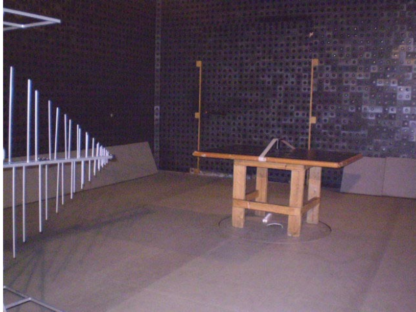
Photograph No.1 Carrier and spurious emissions field strength measurement setup in the anechoic chamber in 30-1000 MHz range
