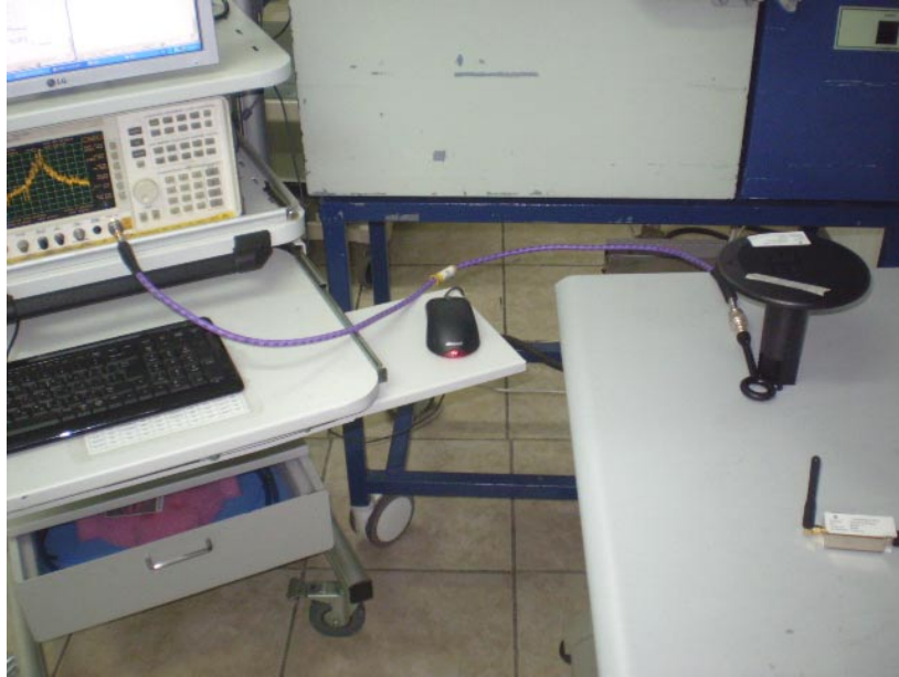
Photograph No.5 Occupied bandwidth, carrier frequency separation, average time of occupancy measurement setup
