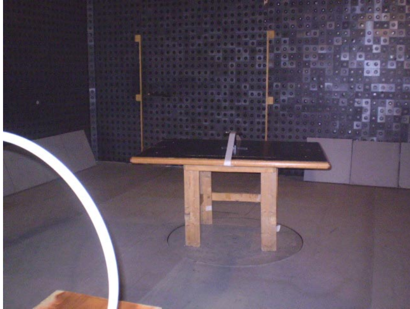
Photograph No.2 Spurious emissions field strength measurement setup in the anechoic chamber below 30 MHz
