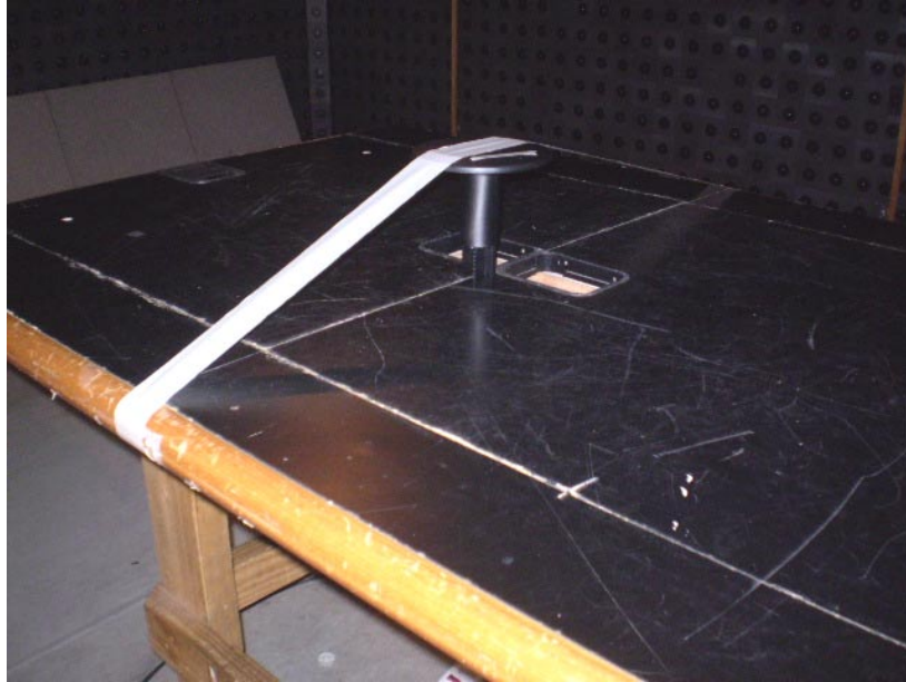
Photograph No.4 Spurious radiated emissions measurement setup in the anechoic chamber, EUT close view
