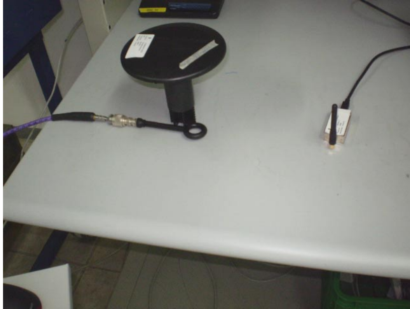
Photograph No.6 Occupied bandwidth, carrier frequency separation, average time of occupancy measurement setup, EUT close view
