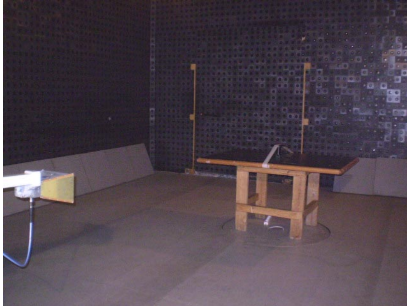
Photograph No.3 Spurious emissions field strength measurement setup in the anechoic chamber above 1000 MHz
