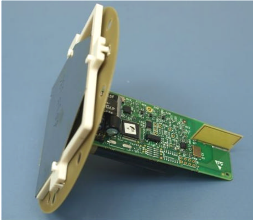
Photograph No.2 Booster 2 water meter internal view
