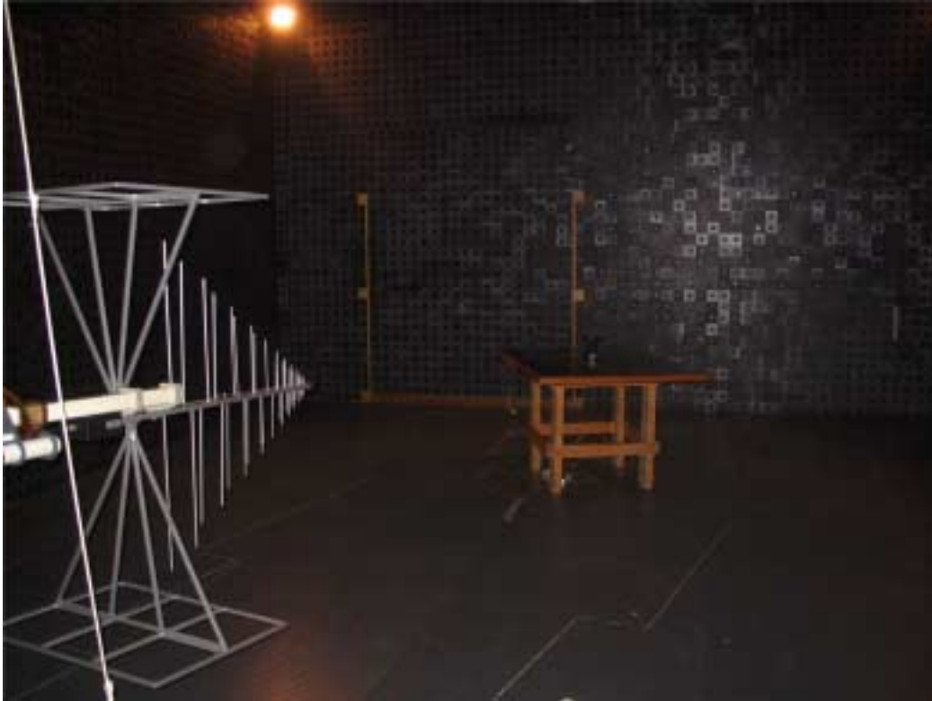
Photograph No.1 Spurious radiated emissions measurement setup in the anechoic chamber with biconilog antenna
