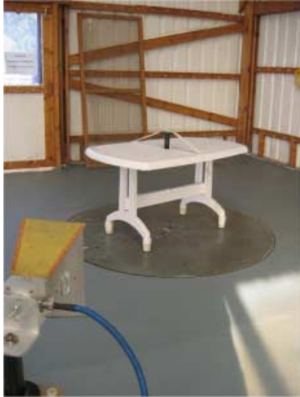
Photograph No.5 Spurious radiated emissions measurement setup at the OATS with double ridged guide antenna
