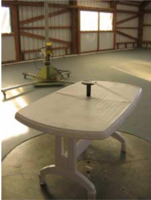
Photograph No.4 Spurious radiated emissions measurement setup at the OATS with double ridged guide antenna
