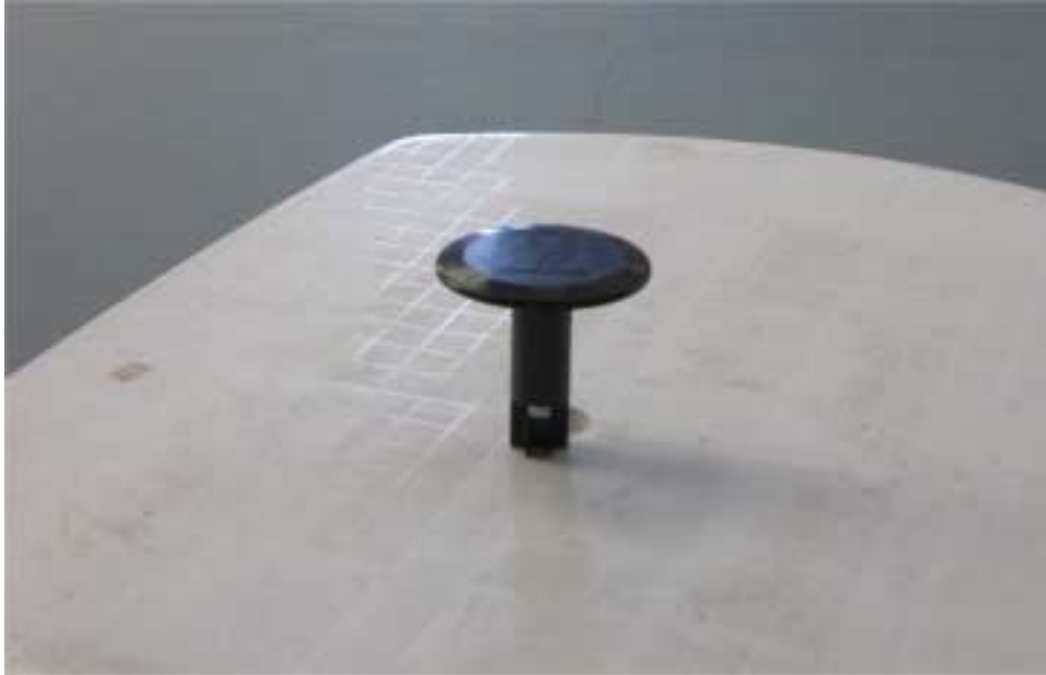
Photograph No.6 Spurious radiated emissions measurement setup at the OATS, EUT close view
