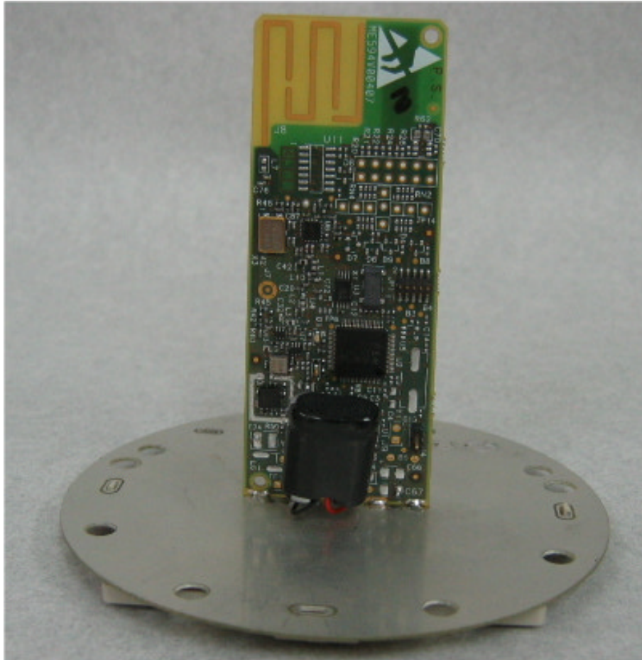
Photograph No.6 Booster water meter PCB general view with printed internal antenna
