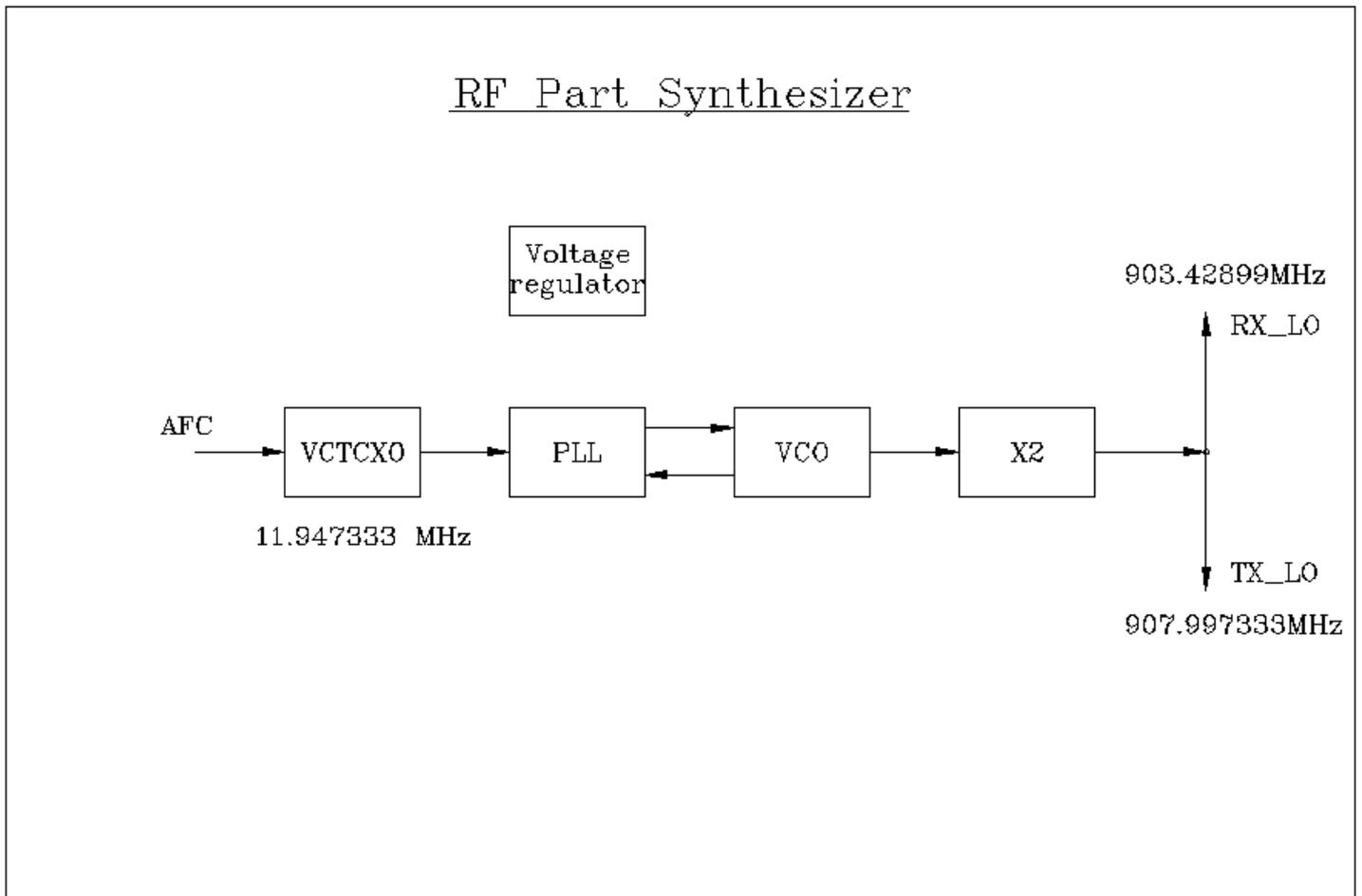
The clock source based on a standard VCTCXO controlled by the CPU. The compensation value is calculated and it is using to control the VCTCXO.
