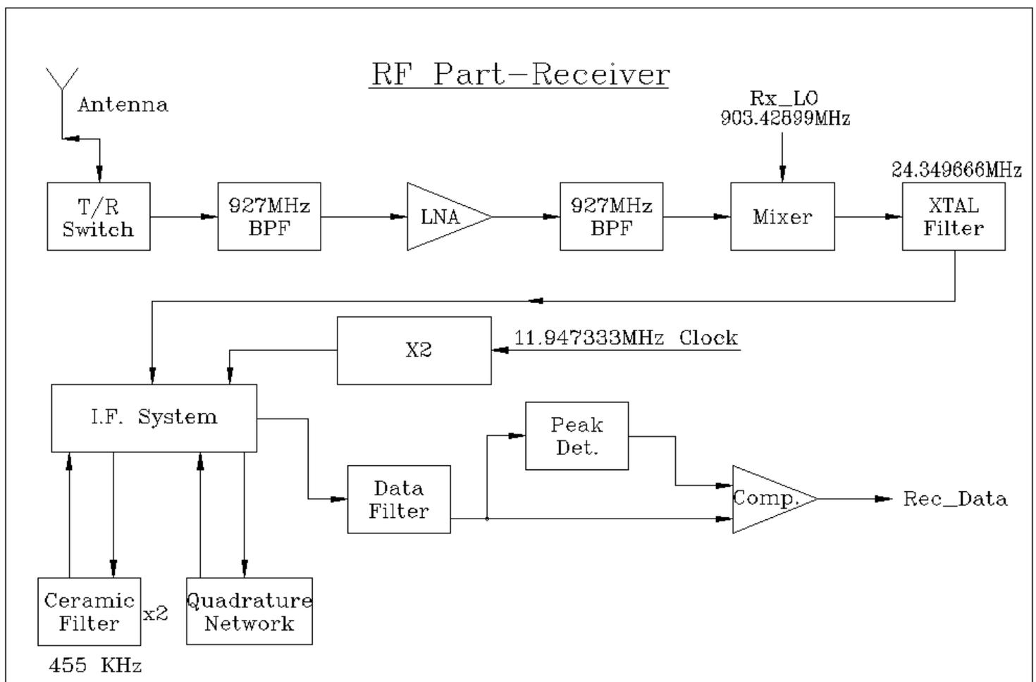
The IF signal enter to crystal filter (BPF) and entered to standard FM discriminator integrated circuit. The output of the discriminator enters to threshold comperator that generates the data signal.
