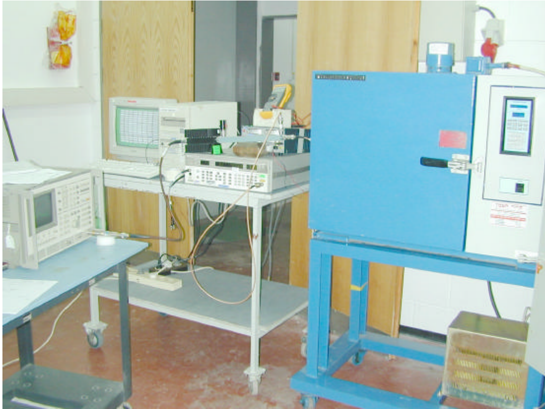
Photograph 4.5.1 Frequency stability test setup
