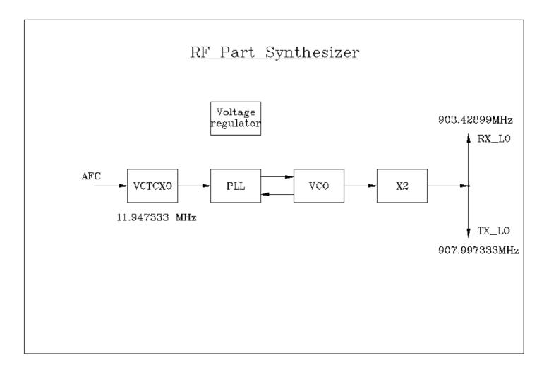
The clock sourse based on a standard VCTCXO controlled by the CPU. The compensation value is calculated and it is using to control the VCTCXO.
