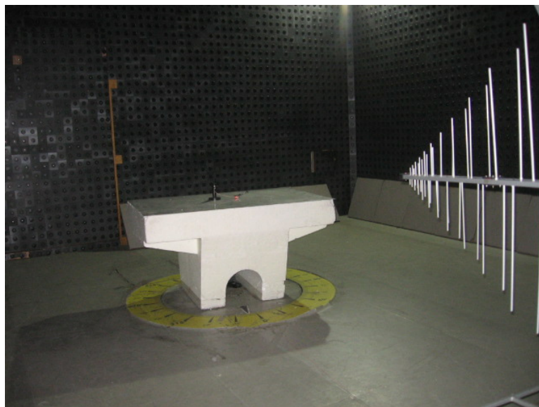
Photograph 8.2.1 Setup for preliminary radiated emission measurements
