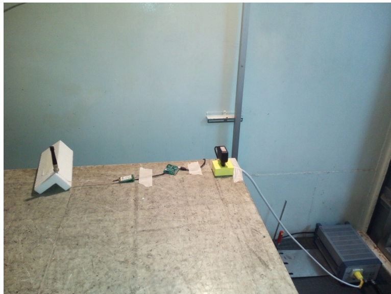
Photograph 8.1.1 Setup for conducted emission measurements
