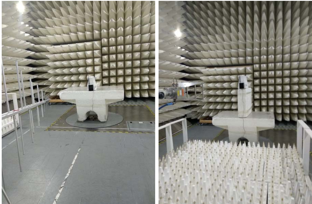
Photograph 8.2.1 Setup for radiated emission measurements, general view
