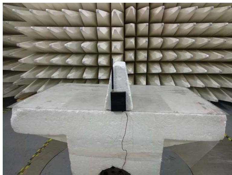
Photograph 8.2.2 Setup for radiated emission measurements, EUT cabling
