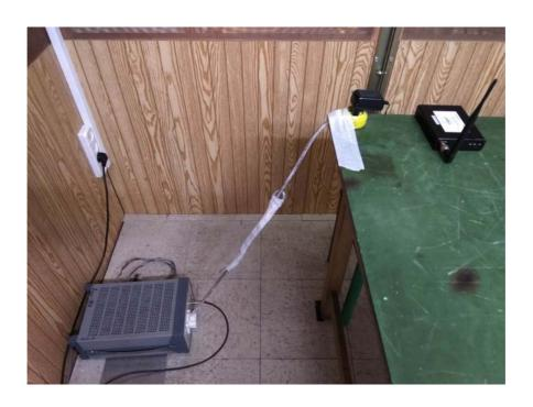
Photograph No.6 Setup for conducted emission measurements on the AC power lines
