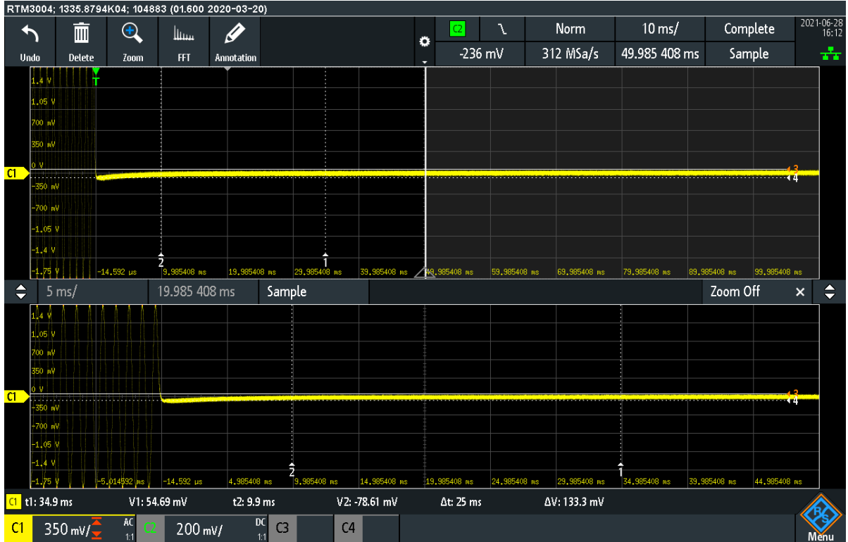
Plot 7.6.8 Transient frequency during power ON test results at high carrier frequency
