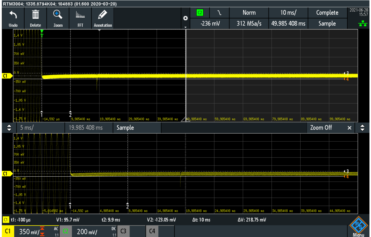
Plot 7.6.4 Transient frequency during power ON test results at mid carrier frequency
