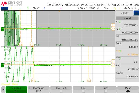
Plot 7.6.5 Transient frequency during power ON test results at high carrier frequency
