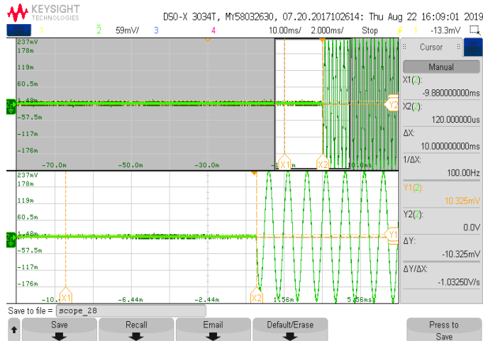
Plot 7.6.4 Transient frequency during power OFF test results at mid carrier frequency
