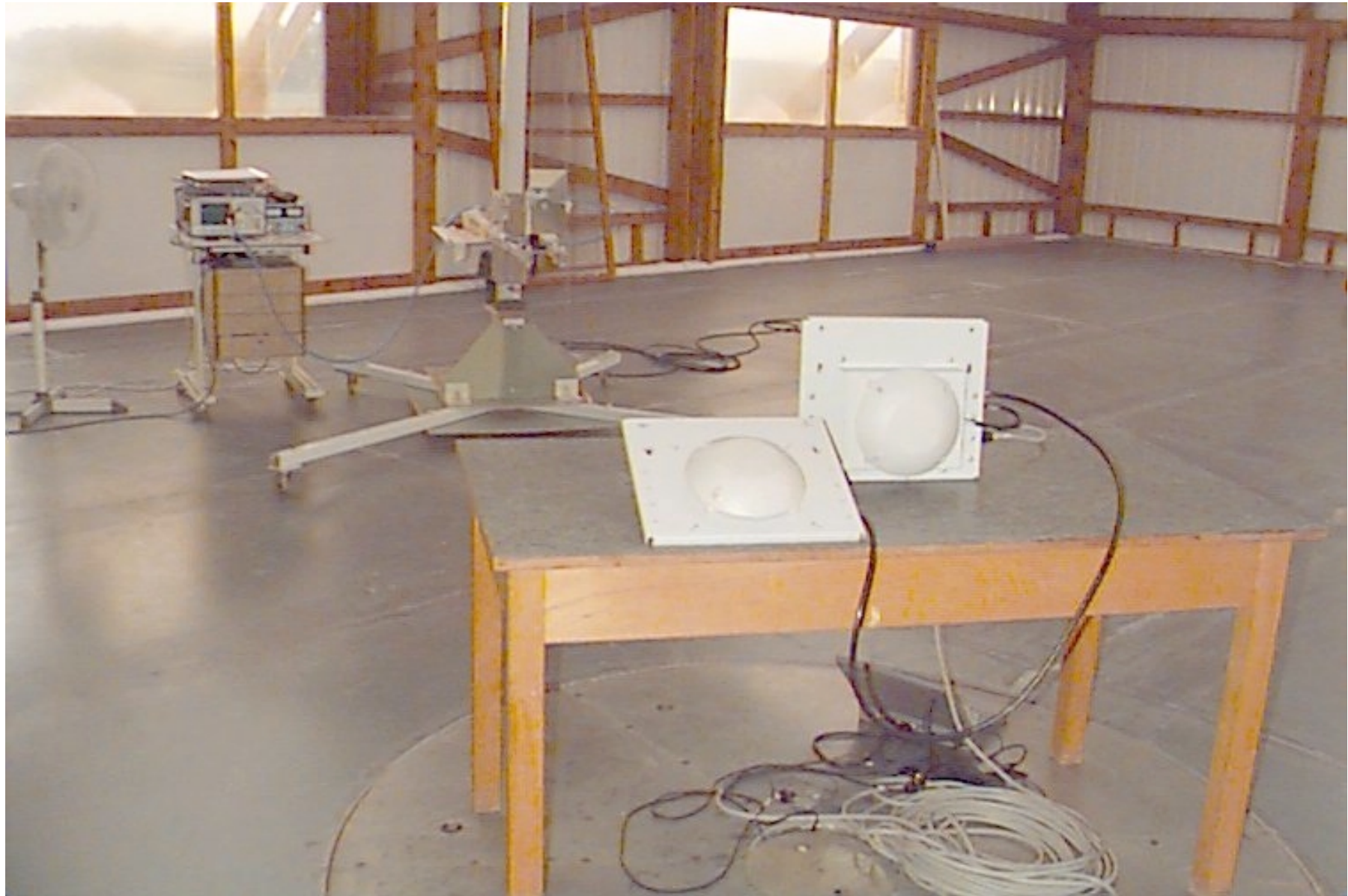
Radiated emission measurements at OATS, above 1 GHz
